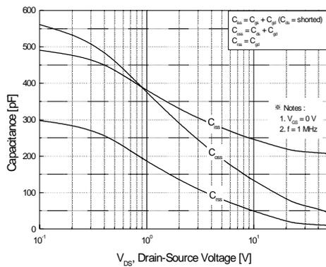
Figure 5. Capacitance Characteristics
