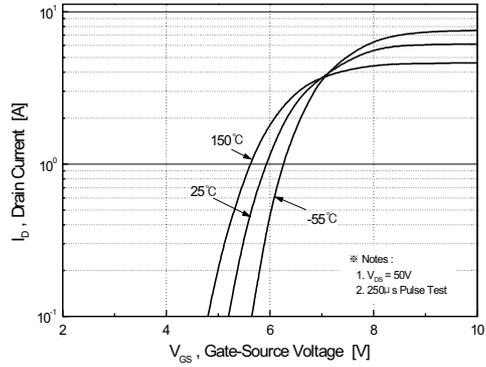
Figure 2. Transfer Characteristics
