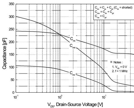
Figure 5. Capacitance Characteristics
