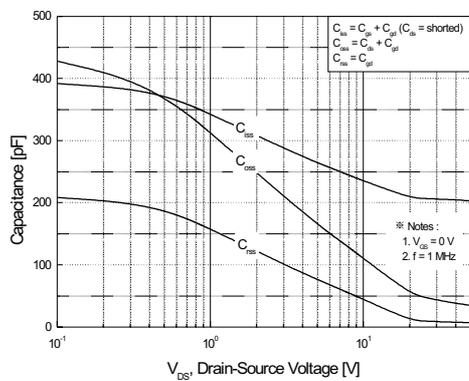
Figure 5. Capacitance Characteristics
