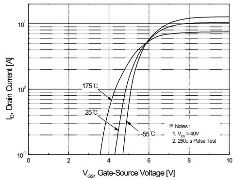
Figure 2. Transfer Characteristics
