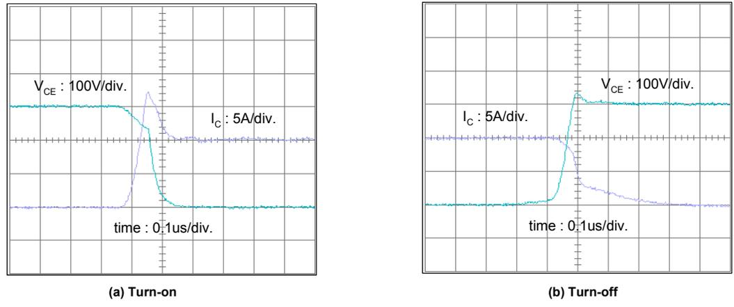
Fig. 5. Experimental Results of Switching Waveforms
