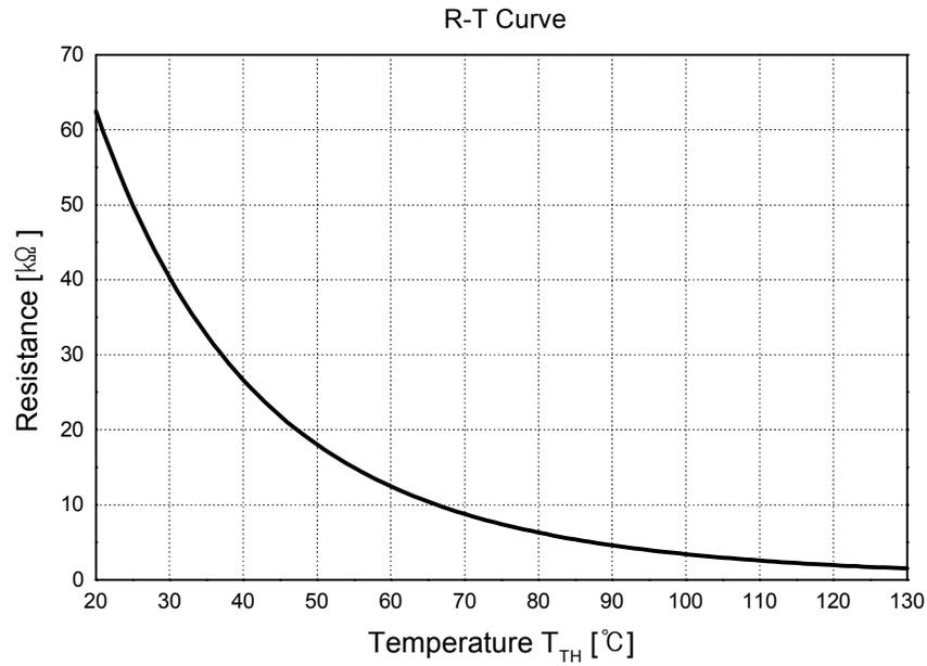
Fig. 6. R-T Curve of The Built-in Thermistor
