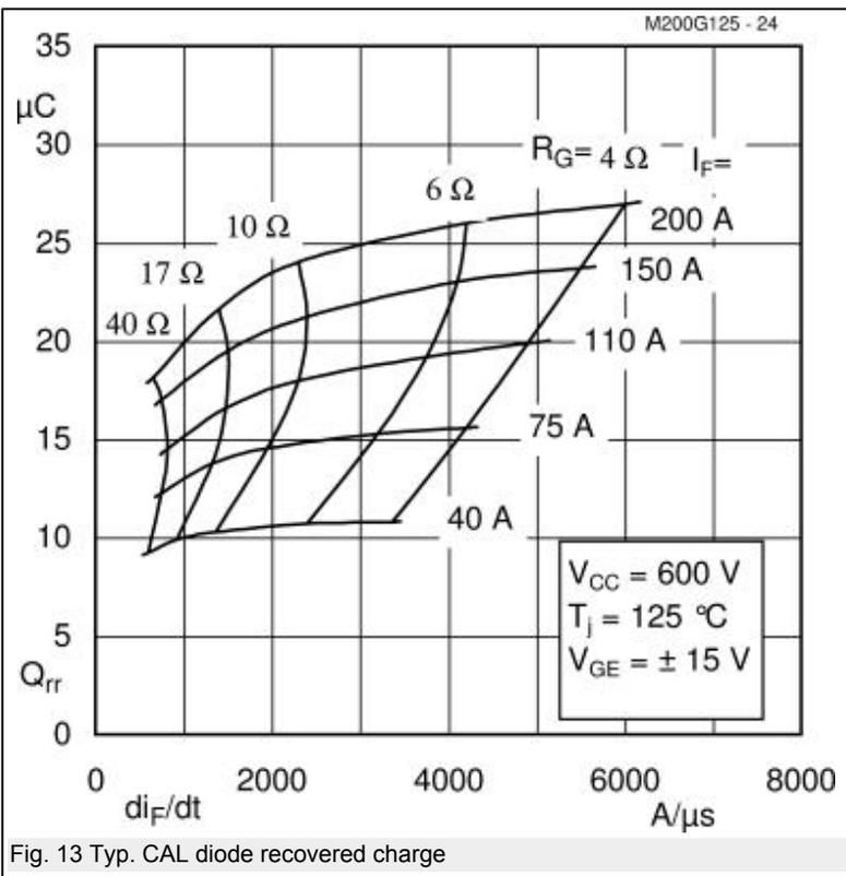
Fig. 13 Typ. CAL diode recovered charge
