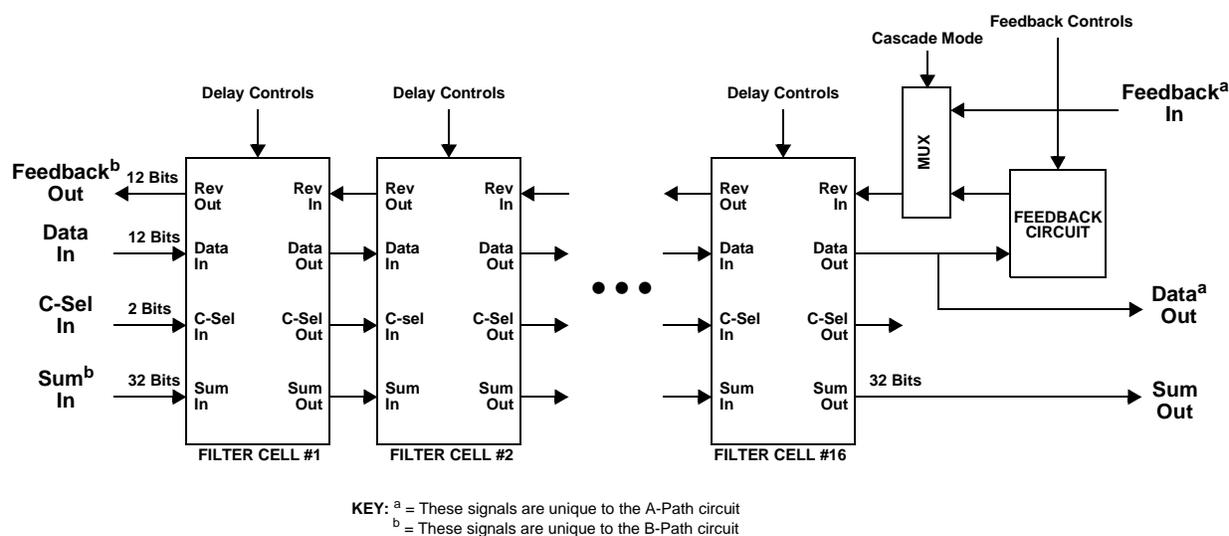
Figure 4. 16 Cell Filter Path Block Diagram
