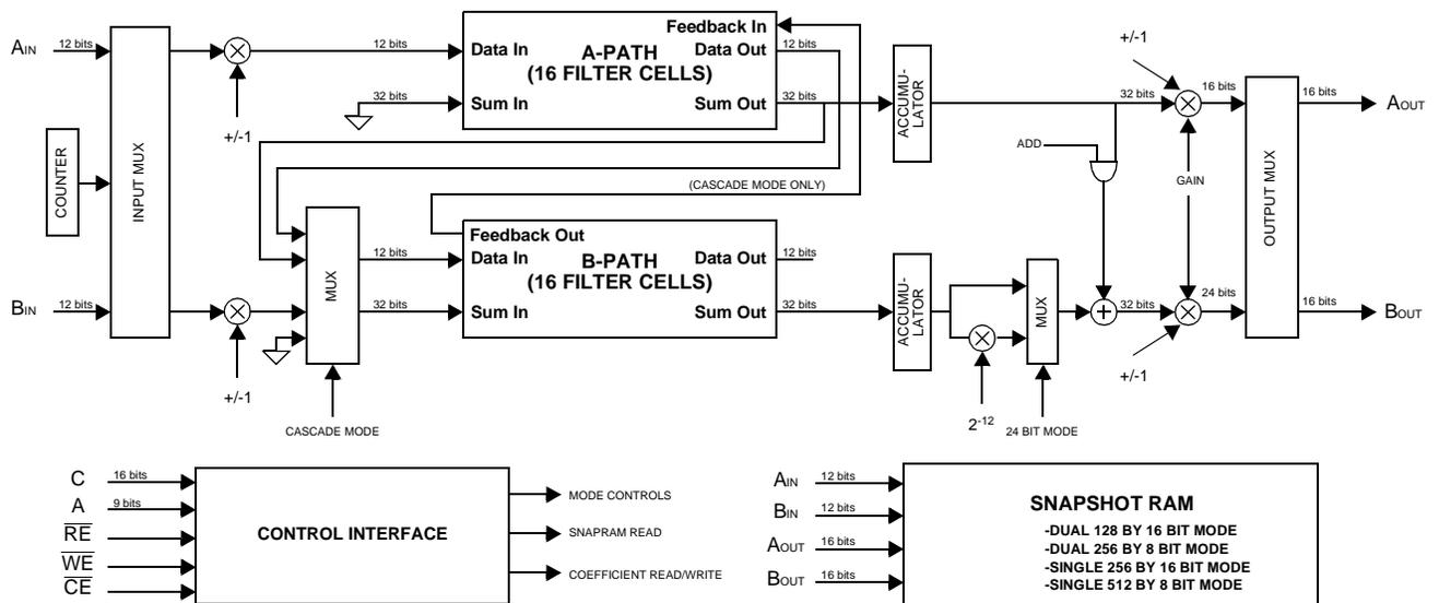
Figure 1. GC2011A Block Diagram
