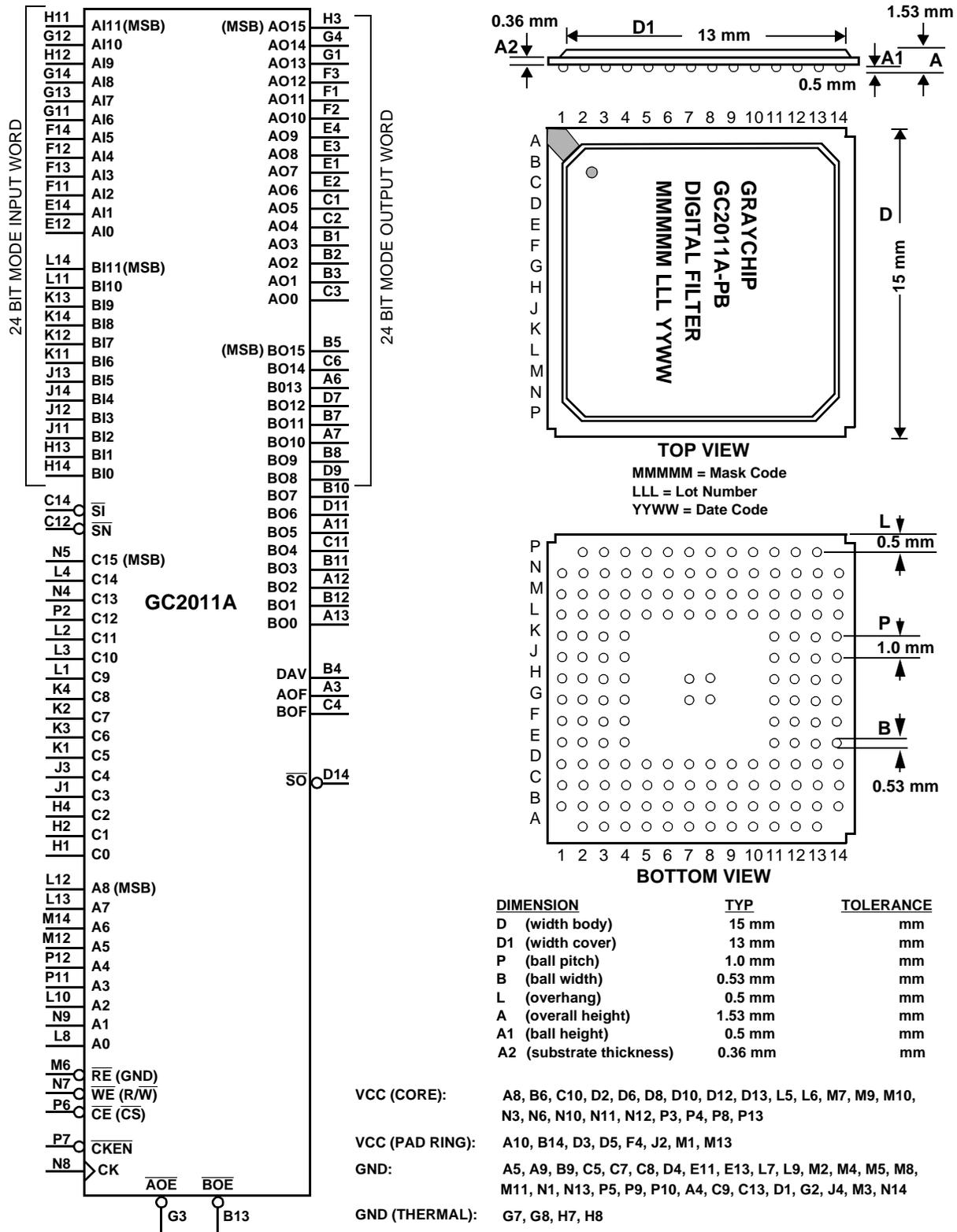
Table 14: Pin Listing For 160 Pin BGA Package (Top View)
