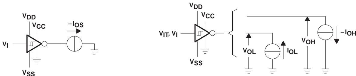
Figure 4. Receiver Test Circuit for  $I_{OS}$
