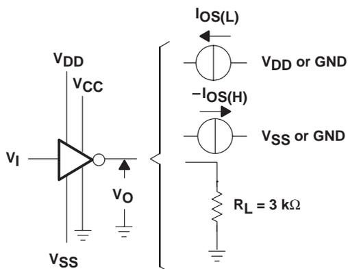
Figure 1. Driver Test Circuit for V<sub>OH</sub>, V<sub>OL</sub>, I<sub>OS(H)</sub>, and I<sub>OS(L)</sub>
