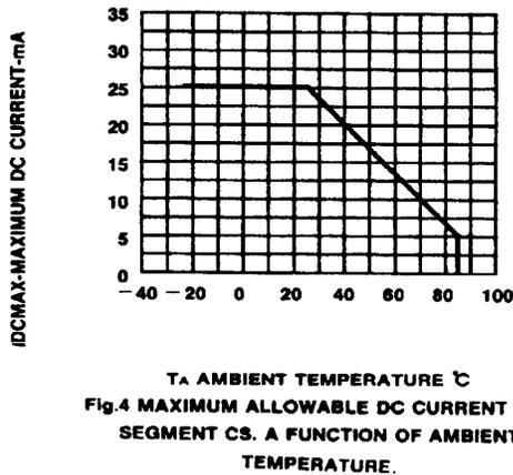
Fig.4 MAXIMUM ALLOWABLE DC CURRENT PER SEGMENT CS. A FUNCTION OF AMBIENT TEMPERATURE.
