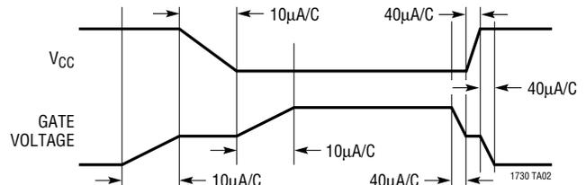
Figure 2. Slew Rate at GATE and V<sub>CC</sub> Pins with the RC Network from GATE to V<sub>CC</sub>
