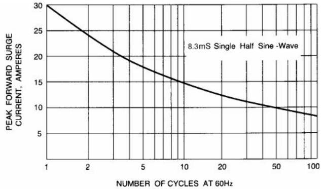
FIG. 2 - MAXIMUM NON-REPETITIVE PEAK FORWARD SURGE CURRENT
