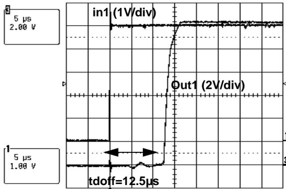
Figure 19. Output ON Delay
