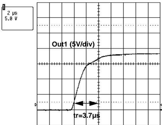
Figure 17. Output Switching Time: Tf
