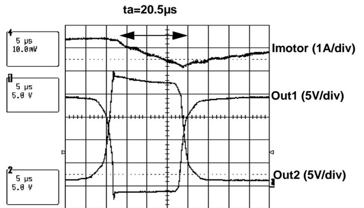
Figure 16. Output Switching Time: Tr
