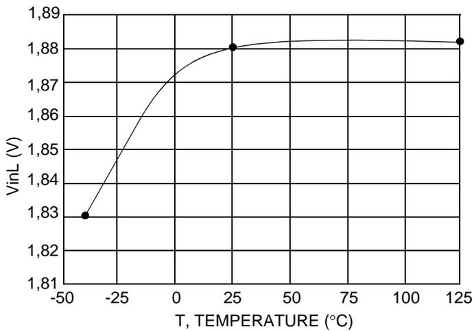
**Figure 9 - High Threshold Input Voltage versus Temperature**
