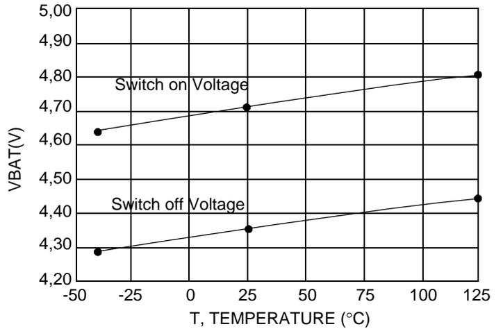
**Figure 8 - Low Threshold Input Voltage versus Temperature**
