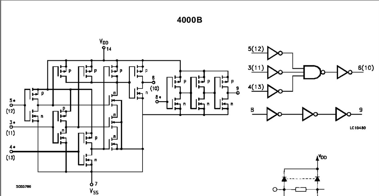
INVERTER AND 1 OF 2 GATES (NUMBERS IN PARANTHESES ARE THERMINAL FOR SECOND GATE)
