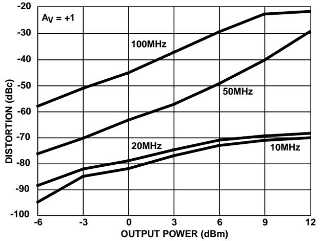
FIGURE 15. 3rd HARMONIC DISTORTION vs  $P_{OUT}$
