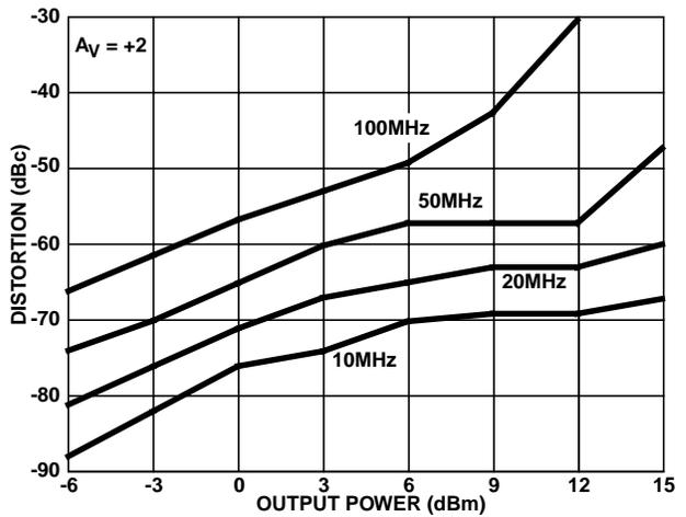
FIGURE 17. 3rd HARMONIC DISTORTION vs  $P_{OUT}$
