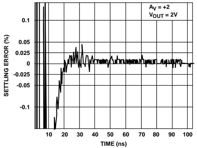
FIGURE 25. SETTLING RESPONSE
