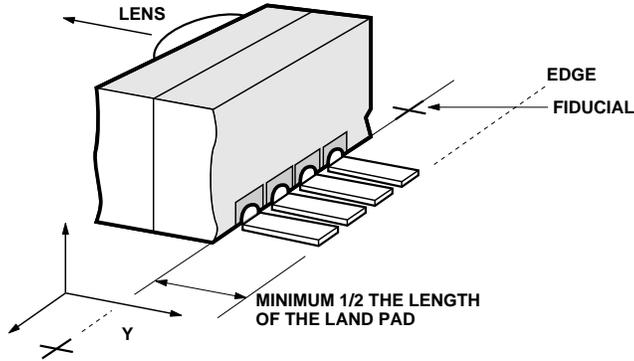
Figure 5. Section of a castellation in Y-axis.
