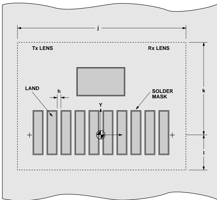
Figure 3. HSDL-3602-007/-037 PCBA-Adjacent land keep-out and solder mask.
