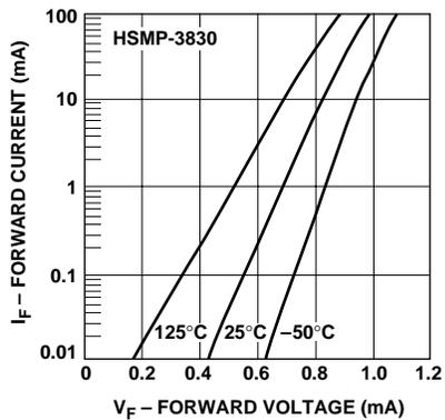
**Figure 16. Forward Current vs. Forward Voltage. HSMP-3830 Series.**
