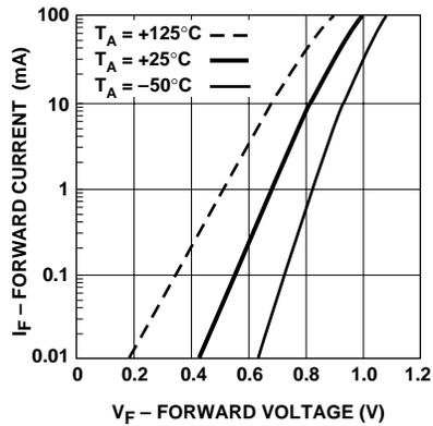
Figure 20. Forward Current vs. Forward Voltage for HSMP-3860.
