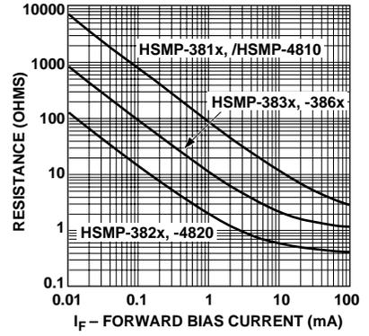
**Figure 3. Resistance at  $25^\circ\text{C}$  vs. Forward Bias Current.**
