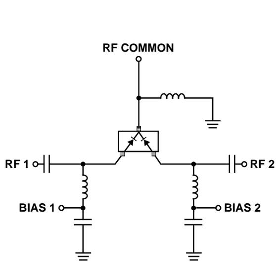
Figure 22. Simple SPDT Switch, Using Only Positive Current.
