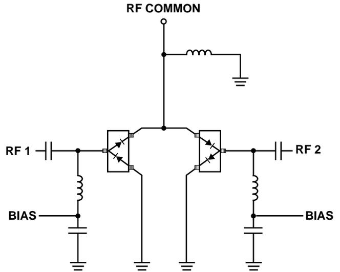
Figure 23. High Isolation SPDT Switch, Dual Bias.
