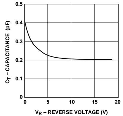
Figure 21. Typical Capacitance vs. Reverse Bias for HSMP-3860.
