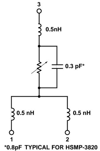
Figure 30. Equivalent Circuit.
