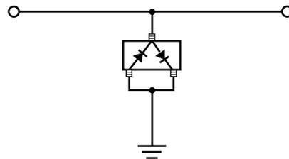
**Figure 28. Power Limiter Using HSMP-3822 Diode Pair.**
