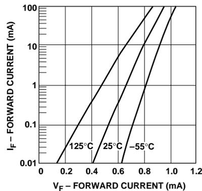
**Figure 17. Forward Current vs. Forward Voltage. HSMP-3880 Series.**
