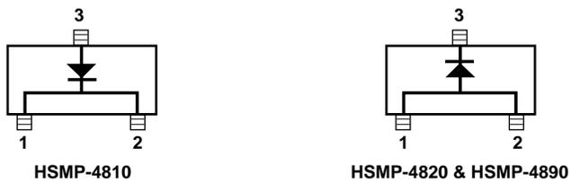
Figure 29. Internal Connections.
