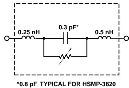
Figure 32. Equivalent Circuit.
