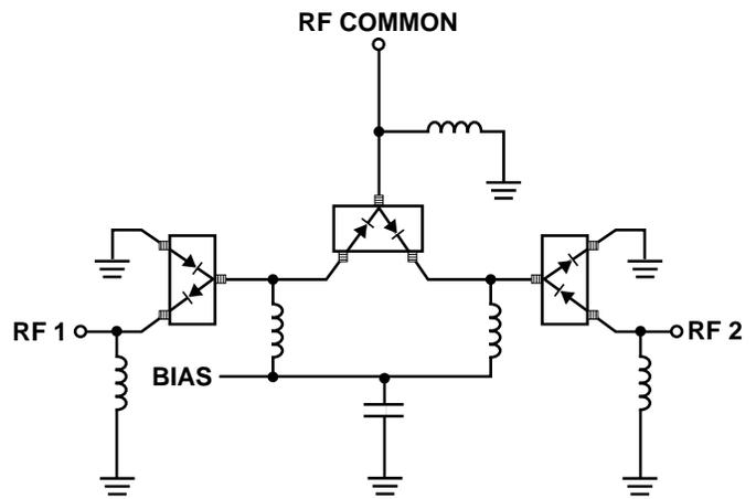
Figure 25. Very High Isolation SPDT Switch, Dual Bias.
