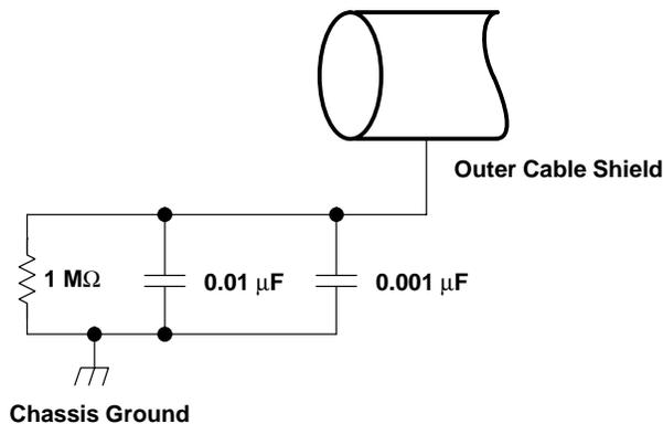
Figure 3–17. Typical Compliant DC Isolated Outer Shield Termination
