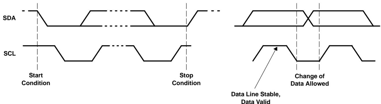
**Figure 3–7. Serial-Bus Start/Stop Conditions and Bit Transfers**
