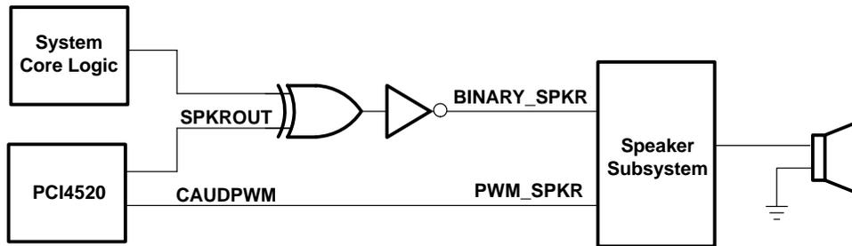
Figure 3–5. Sample Application of SPKROUT and CAUDPWM
