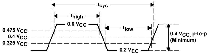
Figure 11–2. CardBus PC Card Clock Waveform
