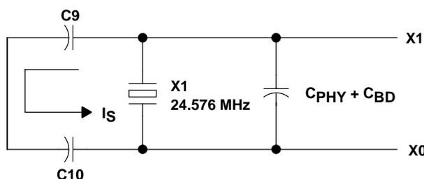
**Figure 3–19. Load Capacitance for the PCI4520 PHY**
