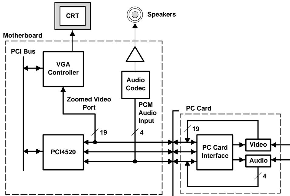
Figure 3–3. Zoomed Video Implementation Using the PCI4520 Device
