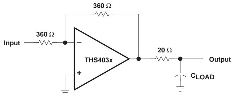
Figure 49. Driving a Capacitive Load
