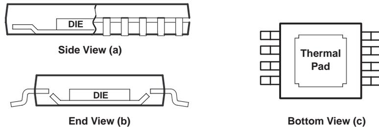
NOTE B: The thermal pad is electrically isolated from all terminals in the package.
