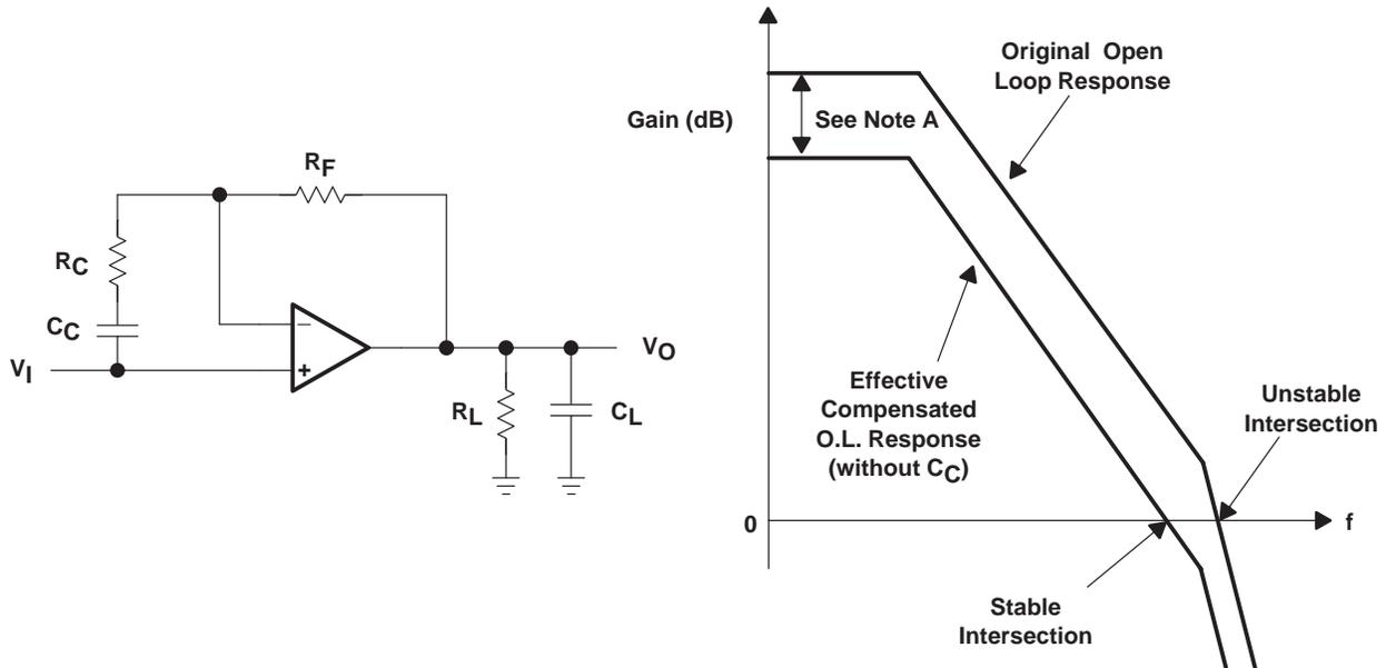
NOTE A: The difference is due to  $1+R_F/R_C$  noise gain.
