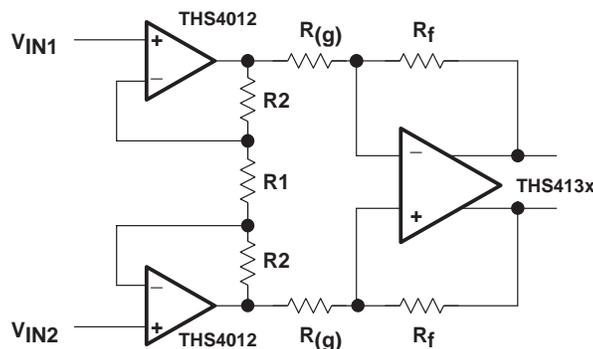
Figure 40. Instrumentation Amplifier
