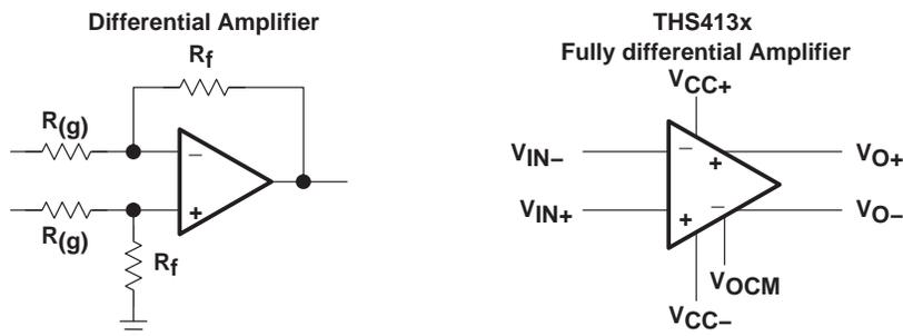
Figure 35. Differential Amplifier Versus a Fully Differential Amplifier
