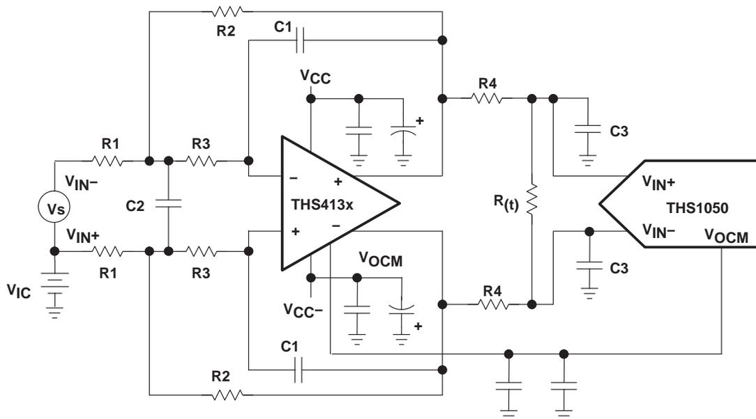
**Figure 34. Antialias Filtering**
