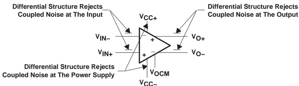
Figure 36. Definition of the Fully Differential Amplifier
