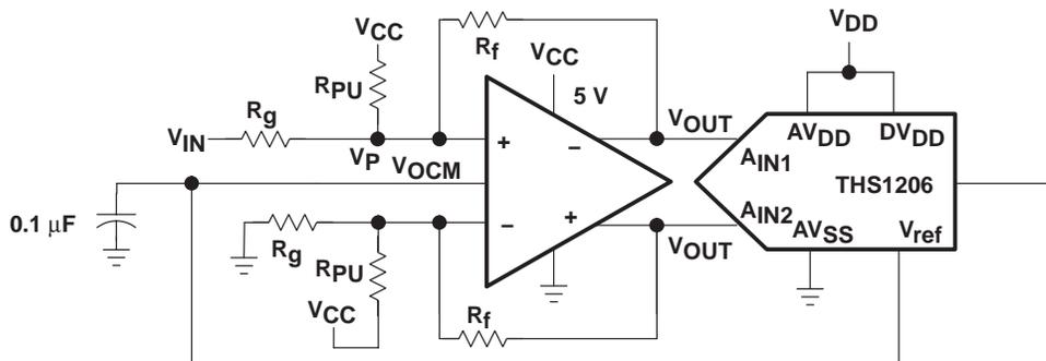
Figure 32. Circuit With Improved Common-Mode Input Voltage
