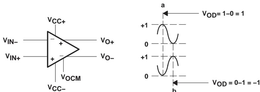
Figure 39. Fully Differential Amplifier With Two 1- $V_{PP}$  Signals
