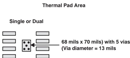
**Figure 28. PowerPAD PCB Etch and Via Pattern**
