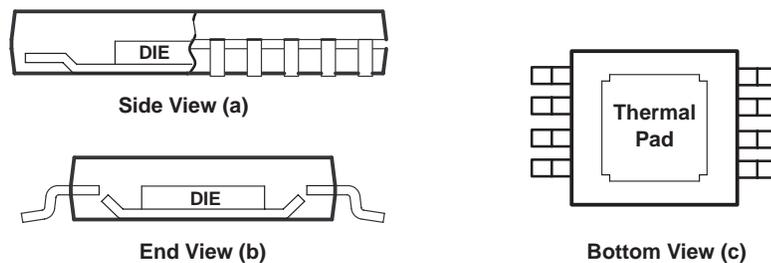
NOTE A: The thermal pad is electrically isolated from all terminals in the package.
