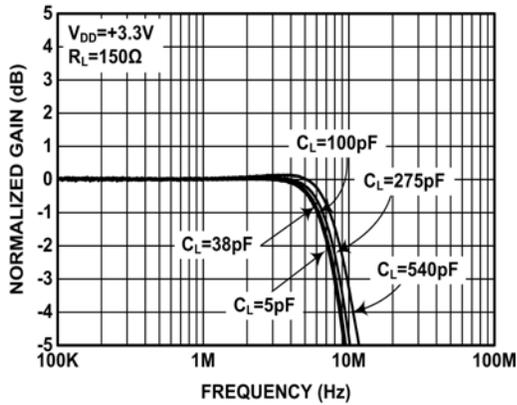
FIGURE 5. GAIN vs FREQUENCY FOR VARIOUS  $C_{LOAD}$
