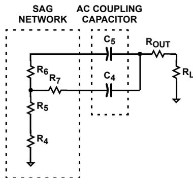
FIGURE 25. SAG NETWORK AND AC COUPLING CAPACITORS
