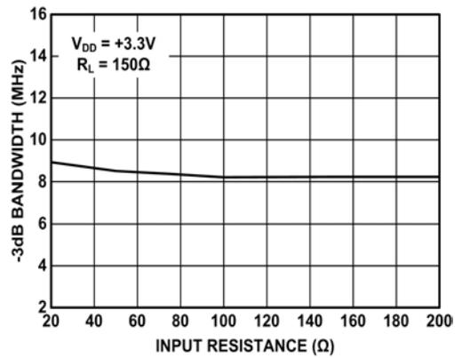
FIGURE 20. -3dB BANDWIDTH VERSUS INPUT RESISTANCE
