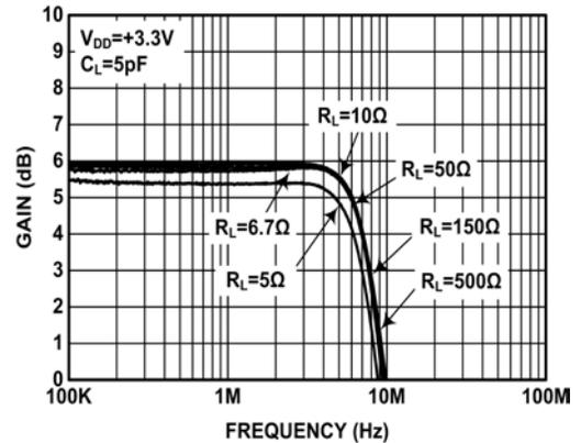
FIGURE 4. GAIN vs FREQUENCY FOR VARIOUS  $R_{LOAD}$
