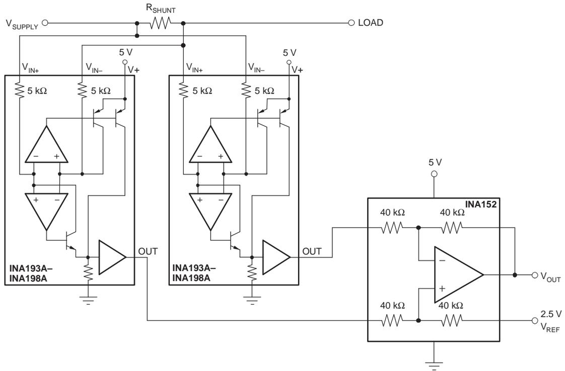
**Figure 5. Bidirectional Current Monitoring**
