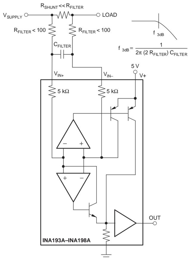
**Figure 2. Input Filter (Gain Error = 1.5% to –2.2%)**
