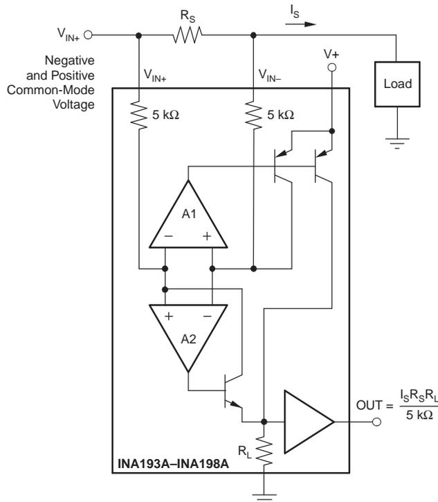
**Figure 3. INA19xA Simplified Circuit Diagram**
