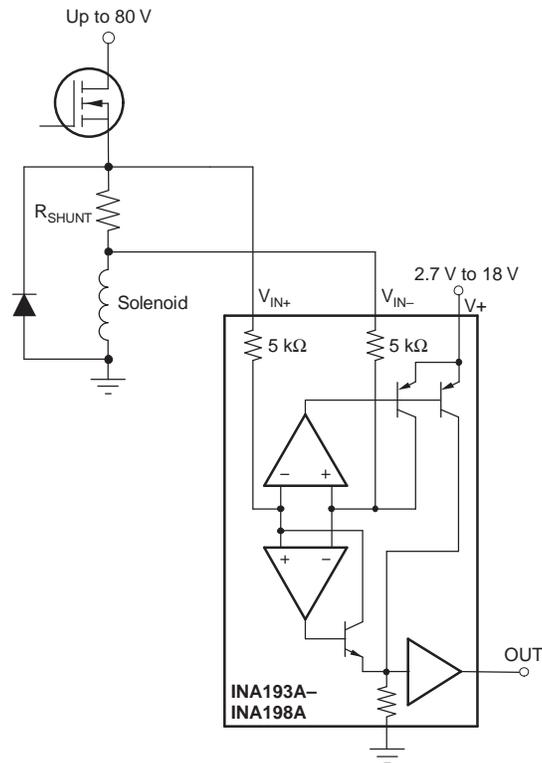
**Figure 6. Inductive Current Monitor Including Flyback**
