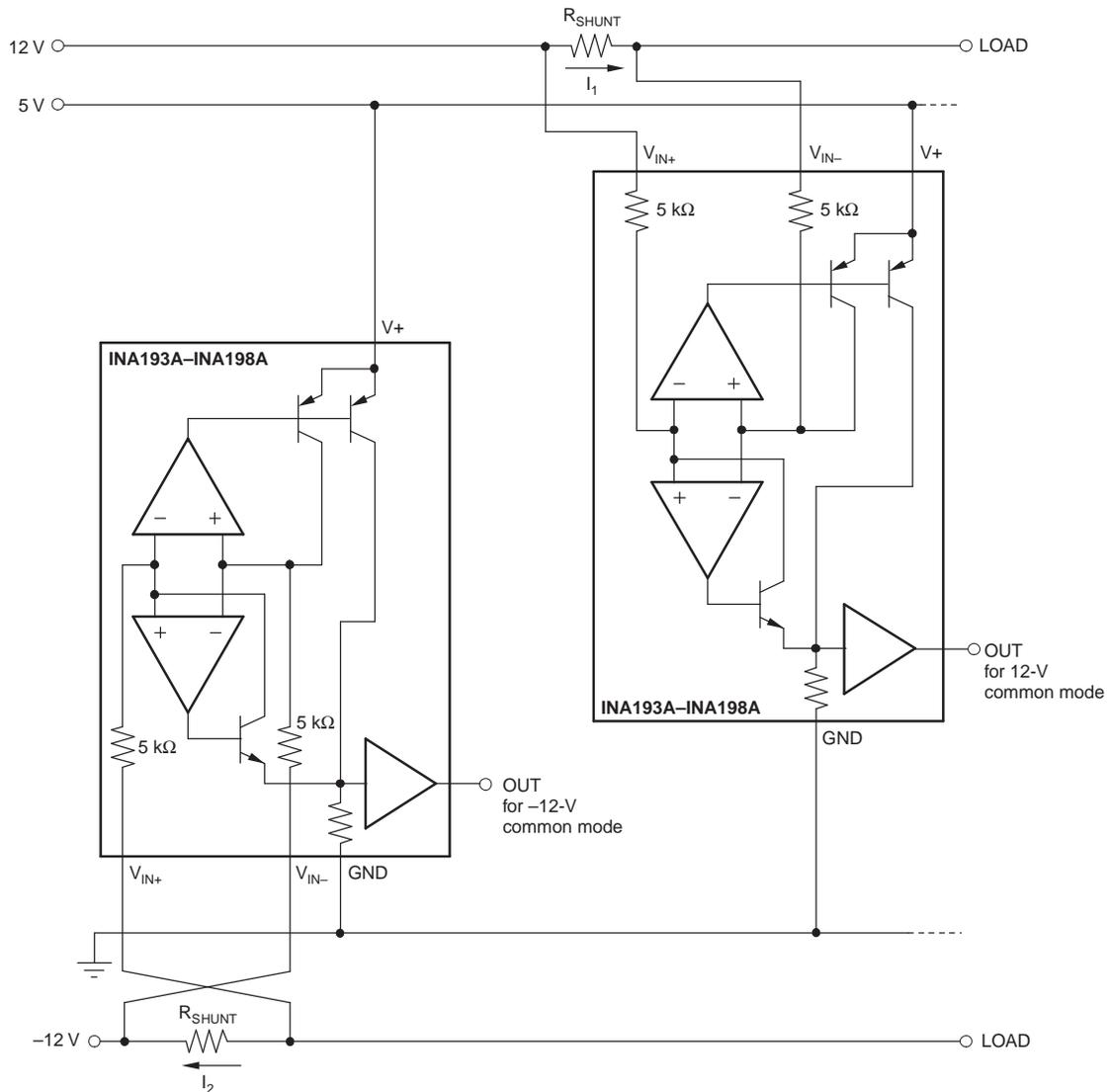
Figure 4. Monitor Bipolar Output Power-Supply Current
