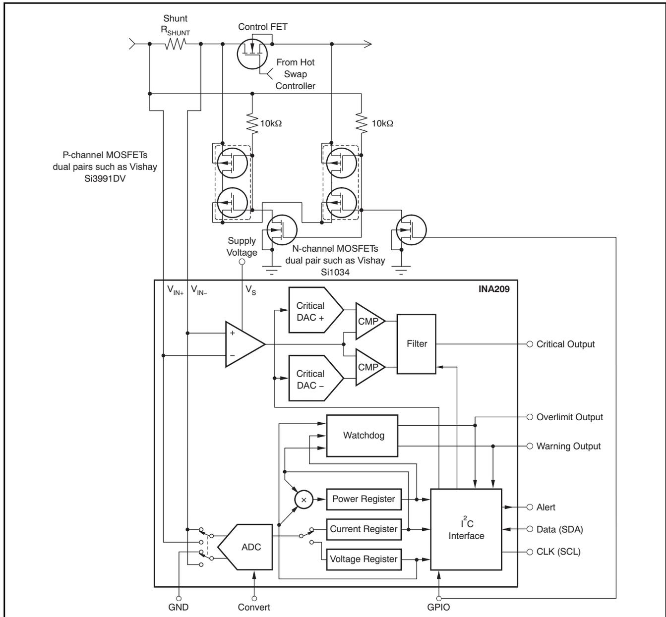
Figure 24. External Circuitry for Additional  $V_{BUS}$  Input
