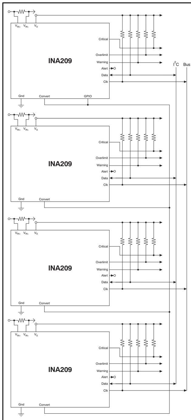
**Figure 23. Multichannel Data Acquisition with Simultaneous Sampling**
