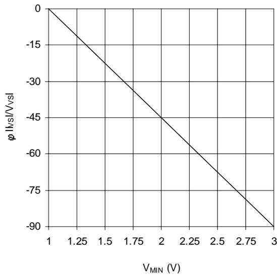
Graph 5.  $\phi I_{vs}/V_{vsI}$  vs  $V_{MIN}$  (IR21592/IR21593)
