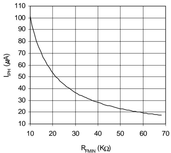
Graph 4. I<sub>IPH</sub> vs R<sub>FMIN</sub> (IR21592/IR21593)
