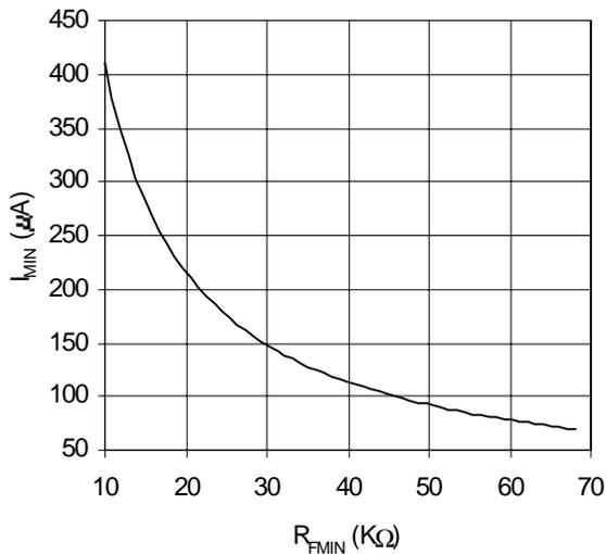
Graph 3. I<sub>MIN</sub> vs R<sub>FMIN</sub> (IR21592/IR21593)
