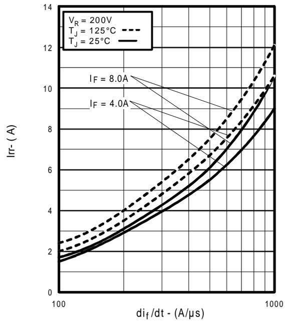
Fig. 15 - Typical Recovery Current vs.  $di_f/dt$
