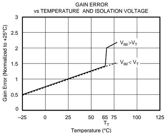
NOTES:  $V_T$  and  $T_T$  approximate the threshold for the indicated gain shift. This is caused by the properties of the optical cavity.
