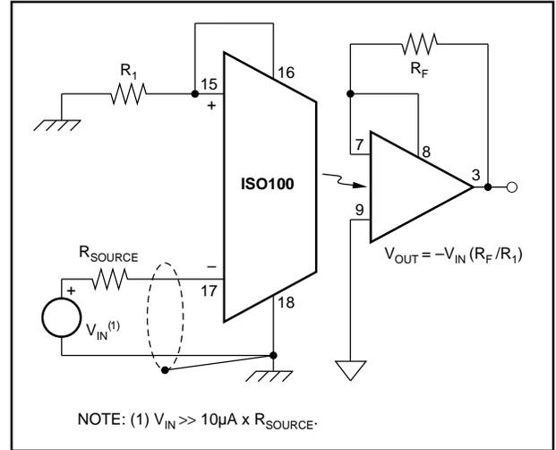
FIGURE 11. Bipolar Inverting.
