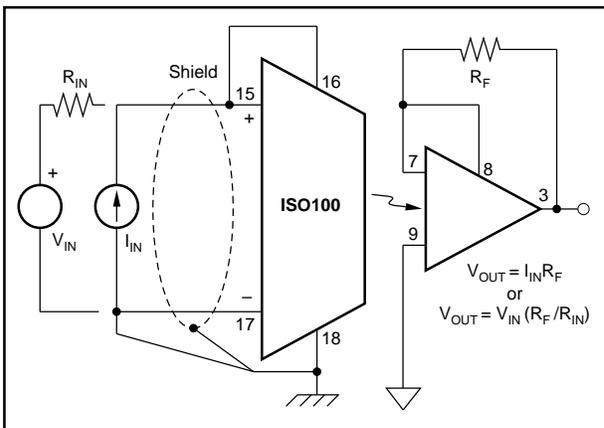
FIGURE 9. Bipolar Noninverting.
