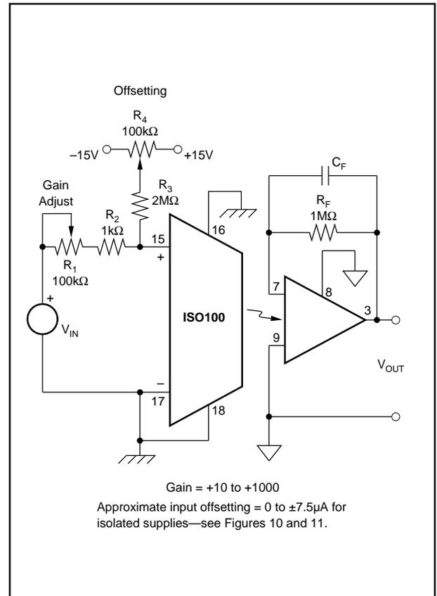
FIGURE 15. Isolated Test Equipment Amplifier (Unipolar with Offsetting).
