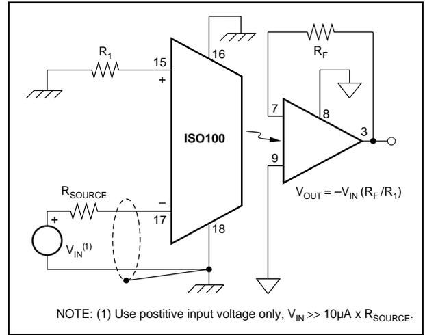
FIGURE 10. Unipolar Inverting.
