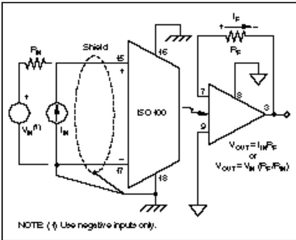
FIGURE 8. Unipolar Noninverting.
