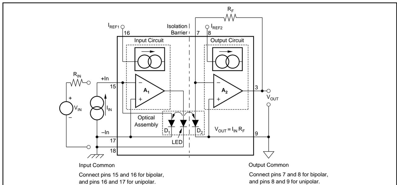
FIGURE 1. Simplified Block Diagram of the ISO100.
