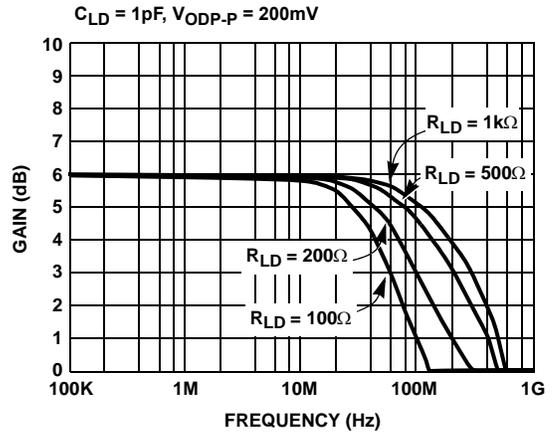
FIGURE 2. SMALL SIGNAL FREQUENCY RESPONSE vs  $R_{LD}$
