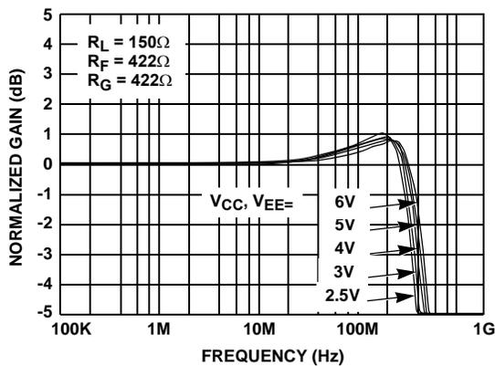
FIGURE 5. FREQUENCY RESPONSE FOR VARIOUS POWER SUPPLY VOLTAGES
