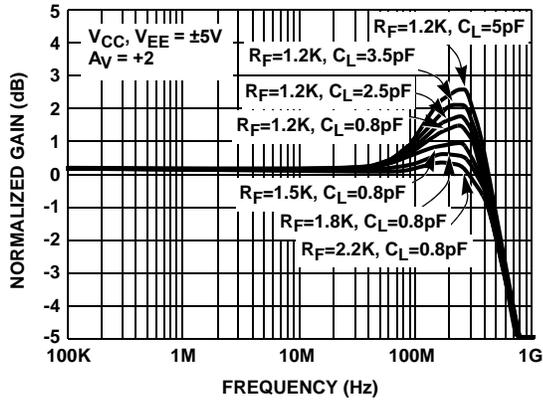
FIGURE 1. FREQUENCY RESPONSE FOR VARIOUS  $R_F$  AND  $C_L$
