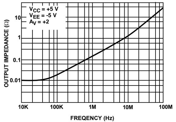
FIGURE 10. OUTPUT IMPEDANCE
