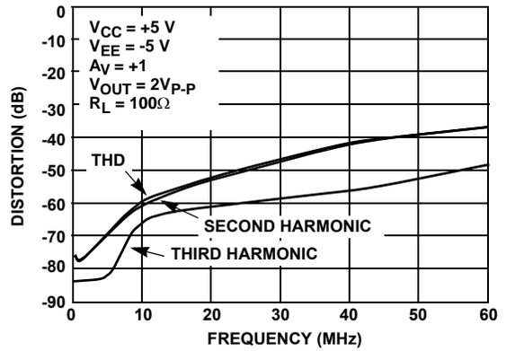
FIGURE 8. DISTORTION vs FREQUENCY ( $A_V = +1$ )
