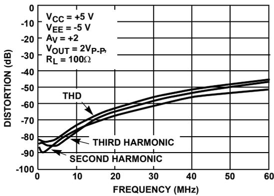
FIGURE 9. DISTORTION vs FREQUENCY ( $A_V = +2$ )
