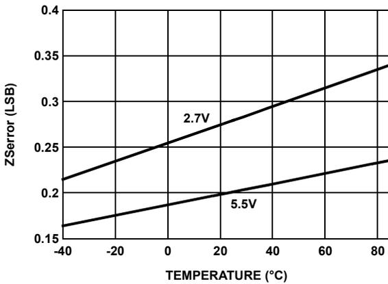
FIGURE 5. ZSerror vs TEMPERATURE FOR 50kΩ (W)
