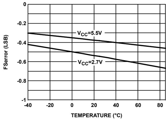
FIGURE 6. FSerror vs TEMPERATURE FOR 50kΩ (W)
