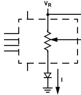
Two terminal variable resistor;
