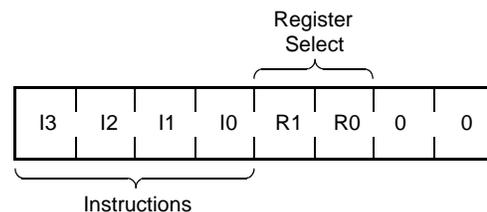
The four high order bits of the instruction byte specify the operation. The next two bits ( $R_1$  and  $R_0$ ) select one of the four registers that is to be acted upon when a register oriented instruction is issued. The last two bits are defined as 0.
