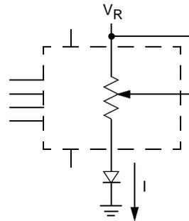
Two terminal Variable Resistor;
