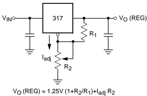
$$V_O (\text{REG}) = 1.25V (1 + R_2/R_1) + I_{\text{adj}} R_2$$
