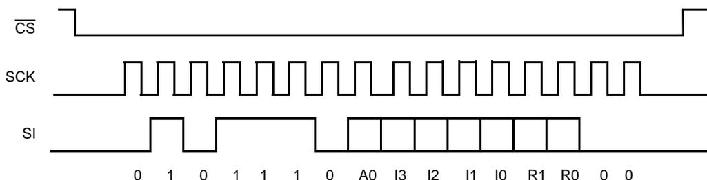
Figure 5. Three-Byte Instruction Sequence (Write)
