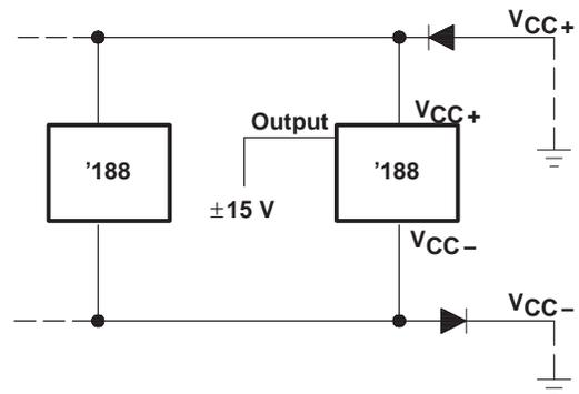
Diodes placed in series with the  $V_{CC+}$  and  $V_{CC-}$  leads protect the SN55188/SN75188 in the fault condition in which the device outputs are shorted to  $\pm 15\text{ V}$ , and the power supplies are at low voltage and provide low-impedance paths to ground.
