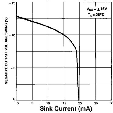
Figure 4. Output voltage swing vs Sink Current (mA)
