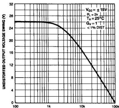
Figure 11. Undistorted Output Voltage Swing vs Frequency
