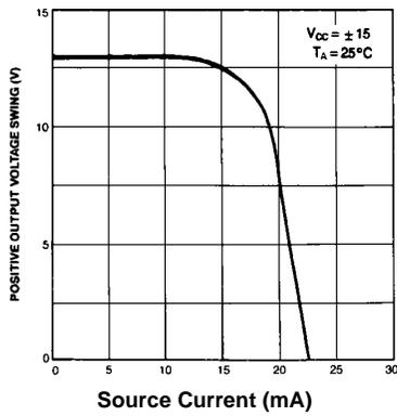
Figure 3. Output voltage swing vs Source Current (mA)
