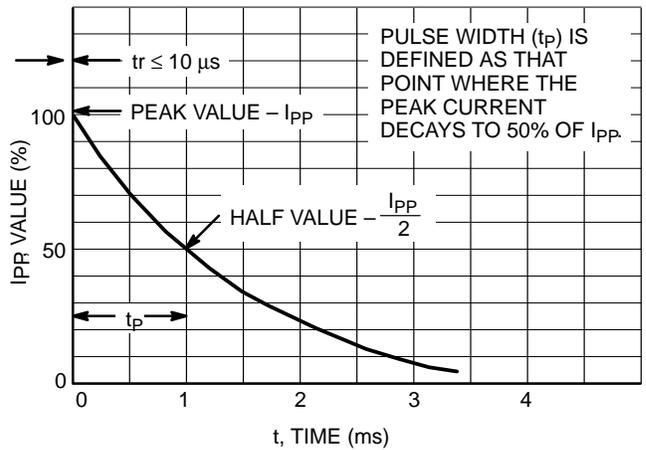
Figure 4. Pulse Waveform
