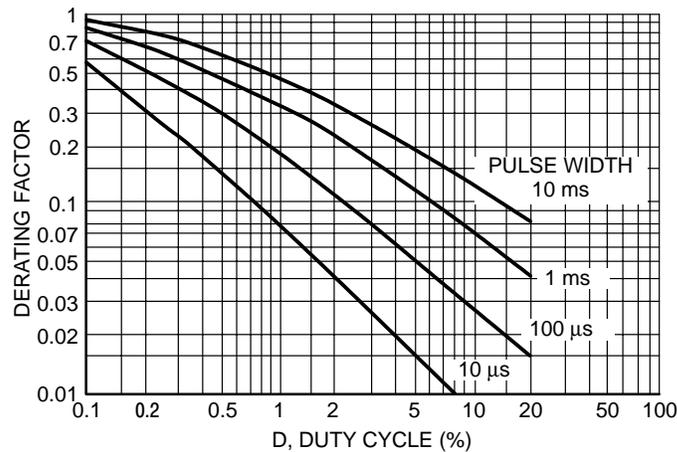
Figure 6. Typical Derating Factor for Duty Cycle
