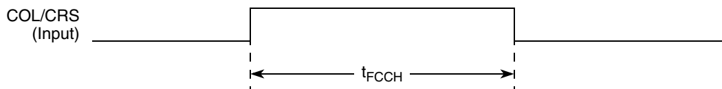
Figure 25. Ethernet Collision AC Timing Diagram (FCC)
