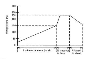
(Note) Complete reflow soldering within 5 seconds at the board surface peak temperature of 240°C or less. The packaging temperature profile varies depending on the board size, type of solder used, and solder thickness.
