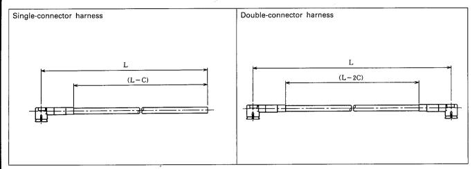
Specify the dimensions from the center of connectors for both single- and double-connector harnesses. Standard dimensional tolerances are as follows:
