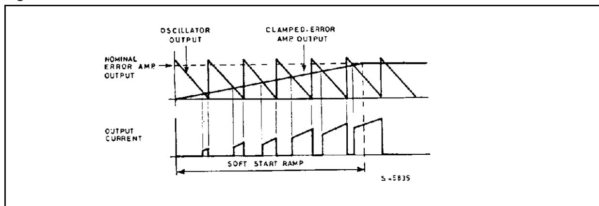
Figure 2. Current limiter waveforms
