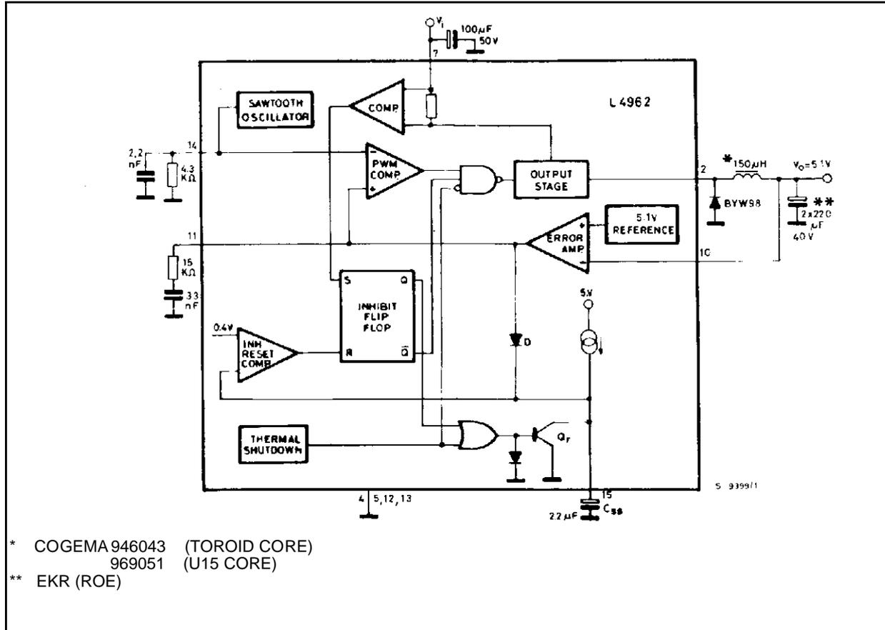
Figure 28. Programmable power supply
