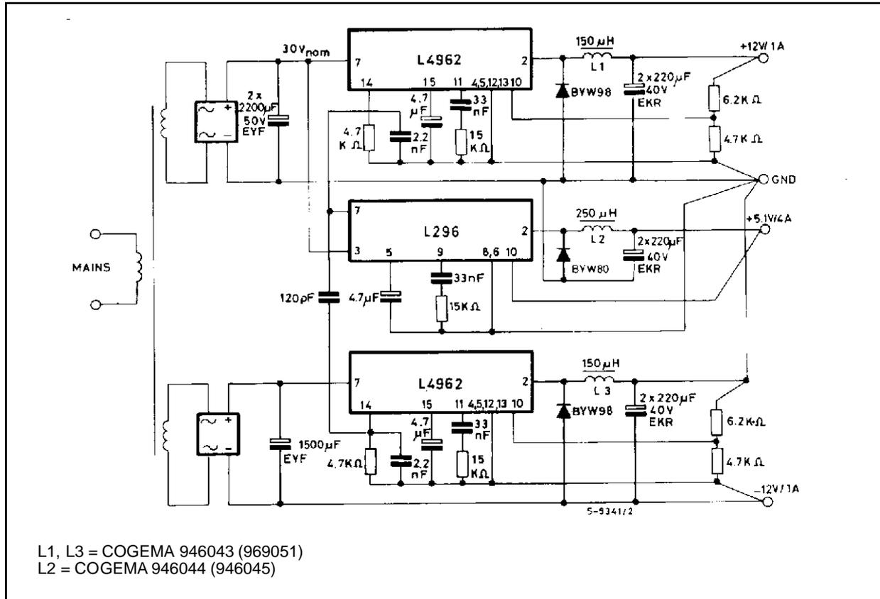
Figure 30. In multiple supplies several L4962s can be synchronized as shown
