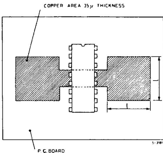
**Figure 33. Maximum dissippable power and junction to ambient thermal resistance vs. side "l"**
