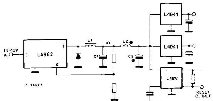
\* L2 and C2 are necessary to reduce the switching frequency spikes when linear regulators are remote from L4962
