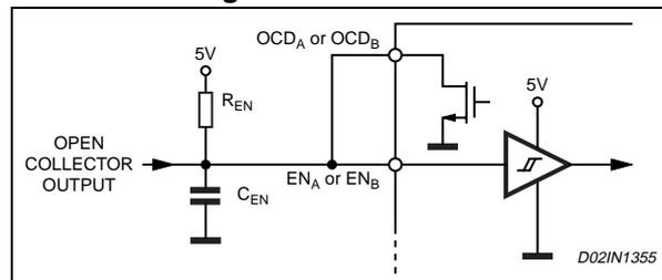
**Figure 6. EN<sub>A</sub> and EN<sub>B</sub> Pins Push-Pull Driving**
