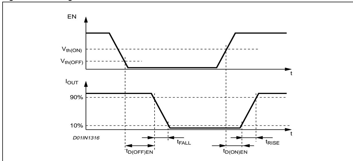
Figure 2. Overcurrent Detection Timing Definition
