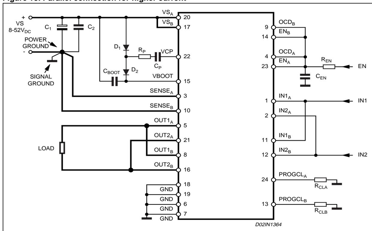
To operate the device in parallel and maintain a lower over current threshold, Half Bridge 1 and the Half Bridge 2 of the Bridge A can be connected in parallel and the same done for the Bridge B as shown in Figure 14. In this configuration, the peak current for each half bridge is still limited by the bond wires for the supply and sense pins so the dissipation in the device will be reduced, but the peak current rating is not increased.
