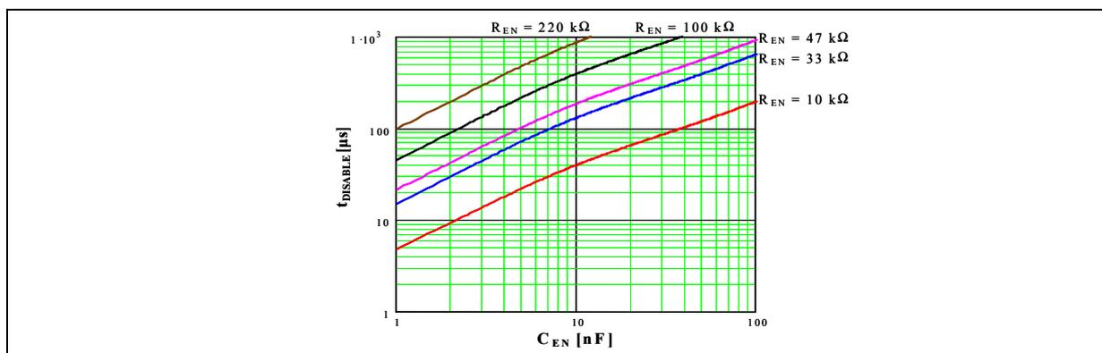
Figure 23. t<sub>DELAY</sub> versus C<sub>EN</sub>.
