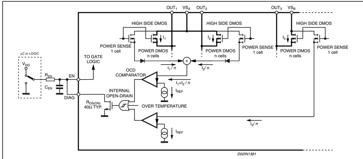
Figure 21 shows the Overcurrent Detection operation. The Disable Time  $t_{DISABLE}$  before recovering normal operation can be easily programmed by means of the accurate thresholds of the logic inputs. It is affected whether by  $C_{EN}$  and  $R_{EN}$  values and its magnitude is reported in Figure 22. The Delay Time  $t_{DELAY}$  before turning off the bridge when an overcurrent has been detected depends only by  $C_{EN}$  value. Its magnitude is reported in Figure 23
