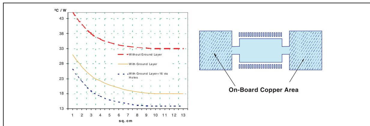
Figure 27. PowerDIP24 Junction-Ambient thermal resistance versus on-board copper area.
