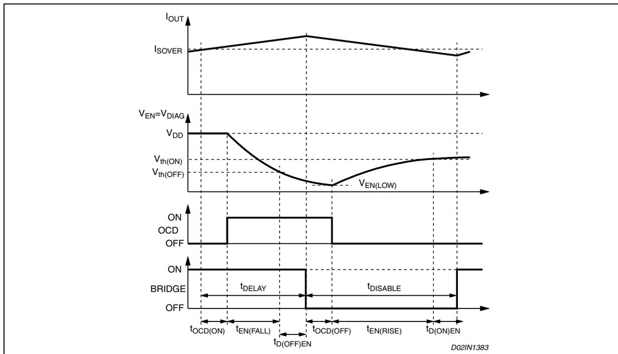
Figure 22. t<sub>DISABLE</sub> versus C<sub>EN</sub> and R<sub>EN</sub>.
