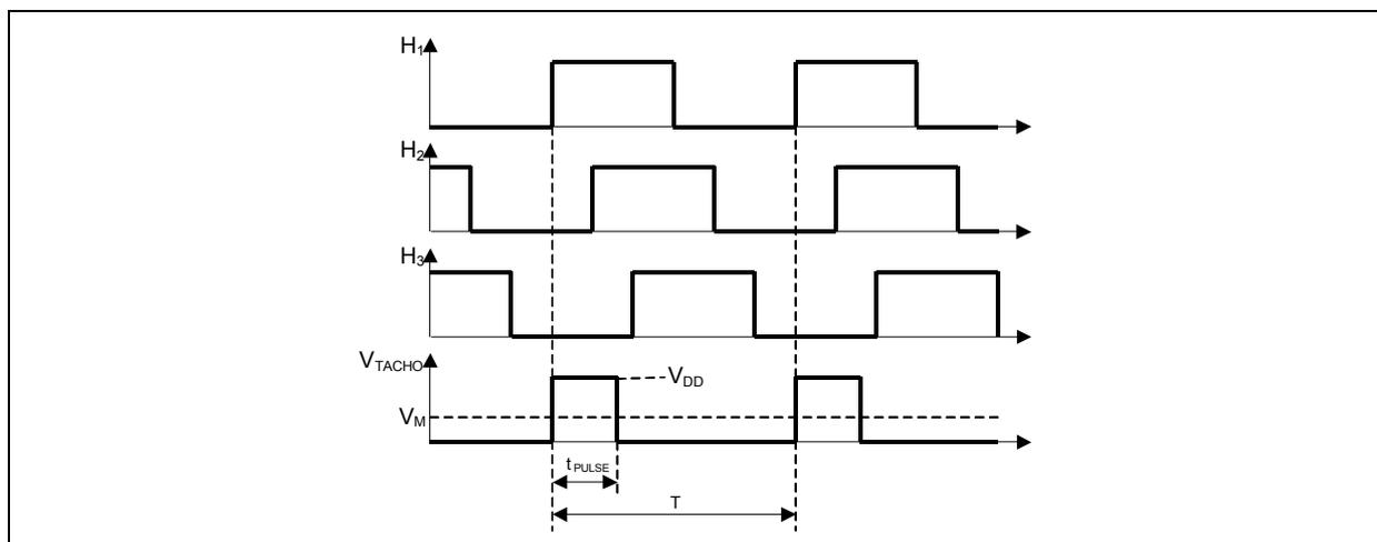
Figure 18. Tachometer Speed Control Loop.
