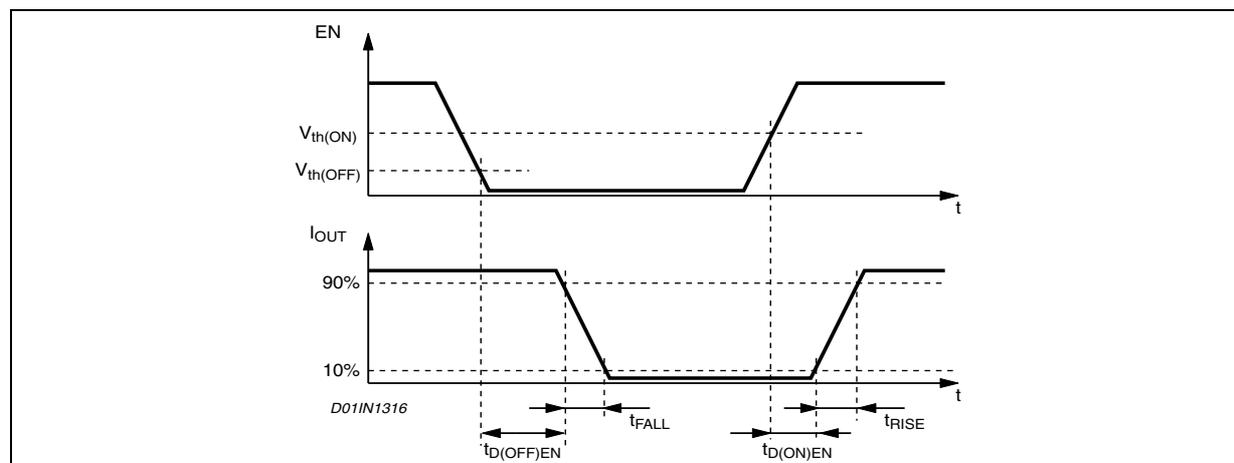
**Figure 5. Overcurrent Detection Timing Definition**
