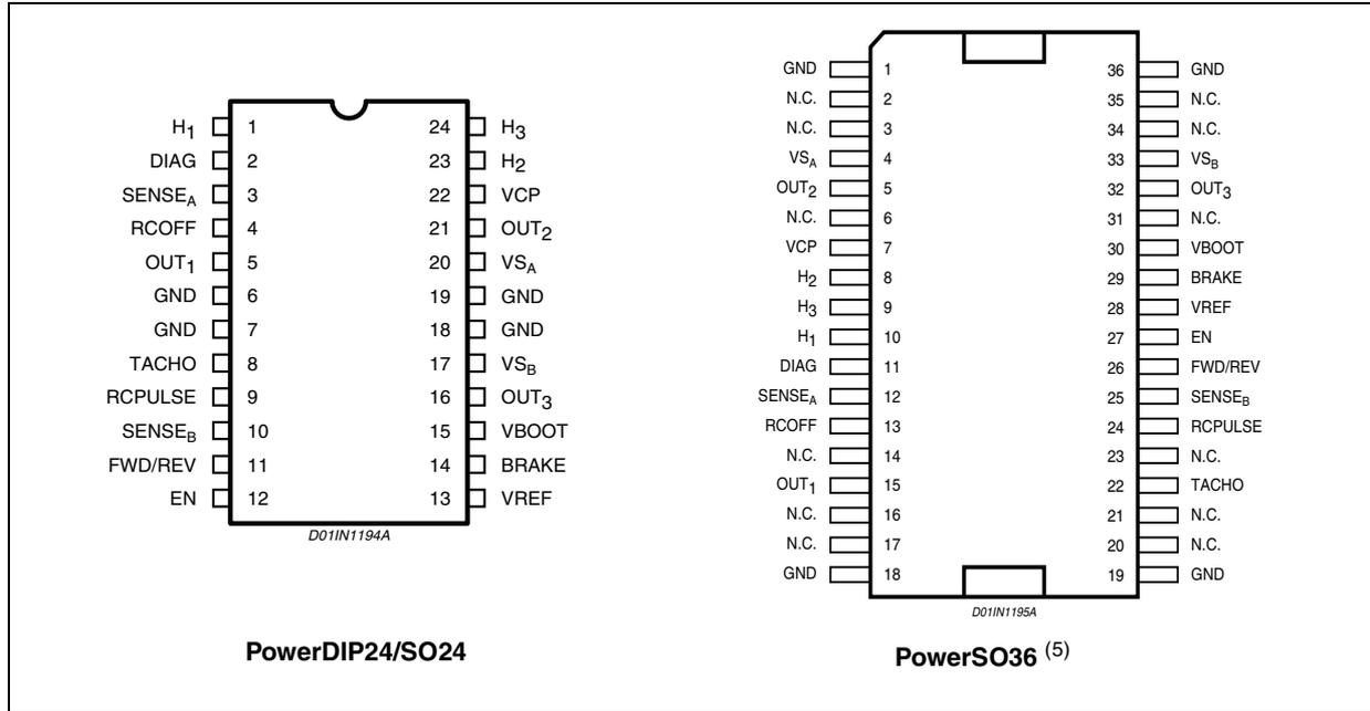
(5) The slug is internally connected to pins 1, 18, 19 and 36 (GND pins).
