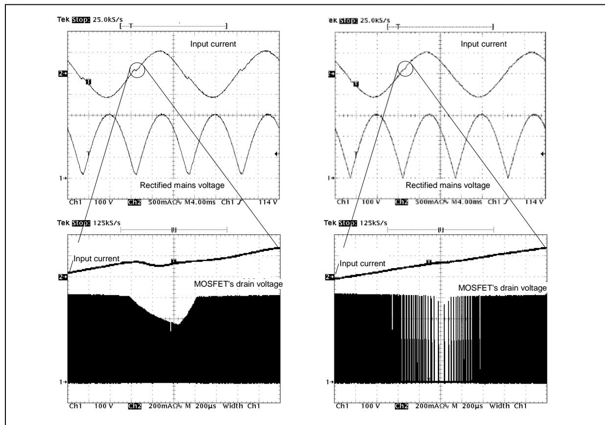
To overcome this issue the circuit embedded in the L6562 forces the PFC pre-regulator to process more energy near the line voltage zero-crossings as compared to that commanded by the control loop. This will result in both minimizing the time interval where energy transfer is lacking and fully discharging the high-frequency filter capacitor after the bridge. The effect of the circuit is shown in figure 23, where the key waveforms of a standard TM PFC controller are compared to those of the L6562.
