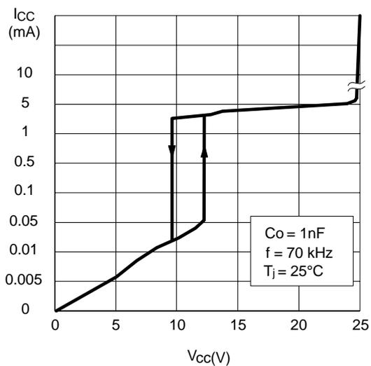
Figure 6. IC consumption vs.  $T_j$
