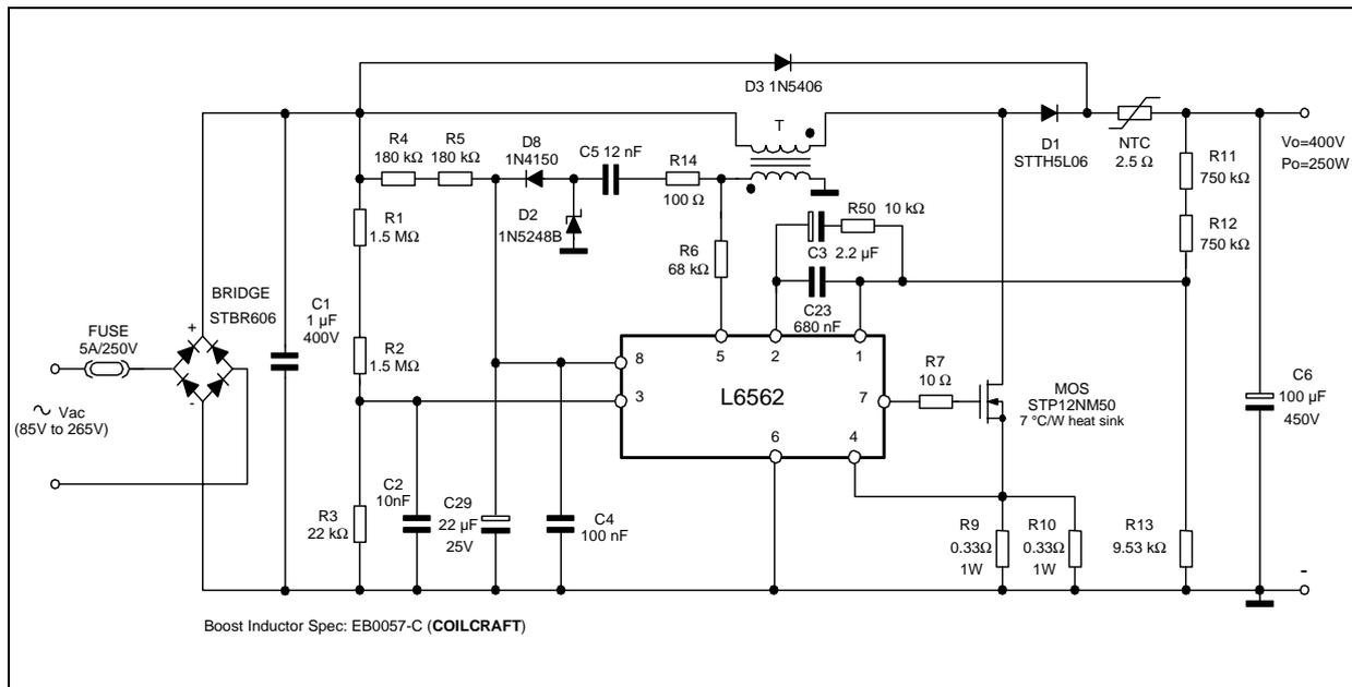
**Figure 24. Demo board (EVAL6562-80W, Wide-range mains): Electrical schematic**
