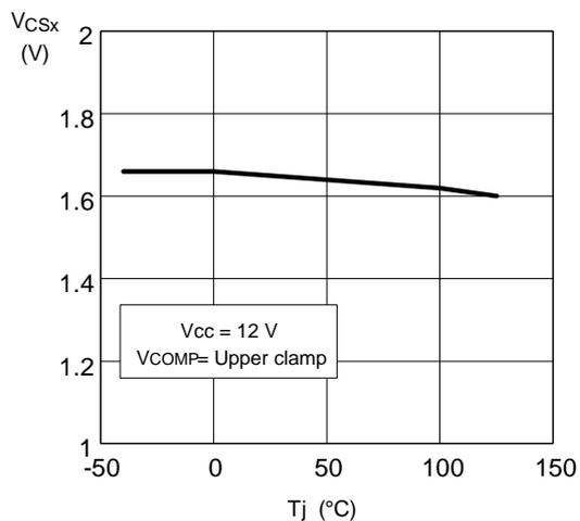
Figure 17. ZCD source capability vs. Tj
