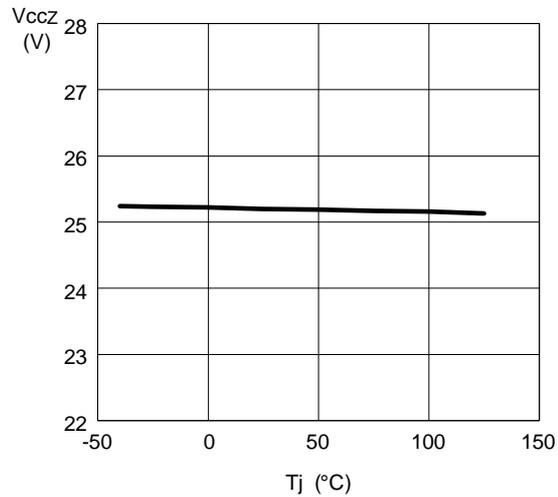
Figure 8. Feedback reference vs.  $T_j$
