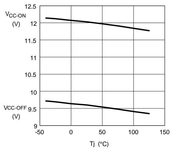
Figure 7.  $V_{CC}$  Zener voltage vs.  $T_j$
