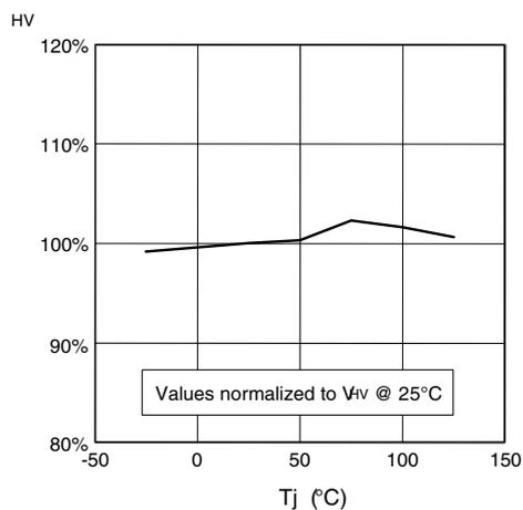
Figure 6. High-voltage generator output (V<sub>CC</sub> charge current) vs. Tj
