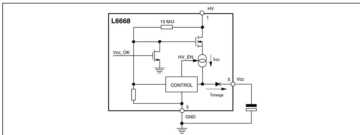
The HV generator is physically located on a separate chip, made with BCD off-line technology able to withstand 700V, controlled by a low-voltage chip, where all of the control functions reside.
