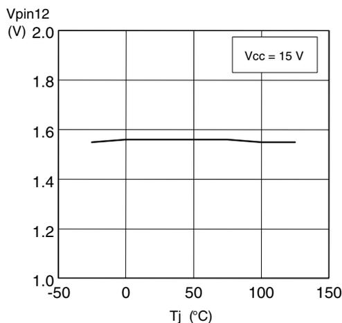
Figure 18. Oscillator ramp vs. Tj
