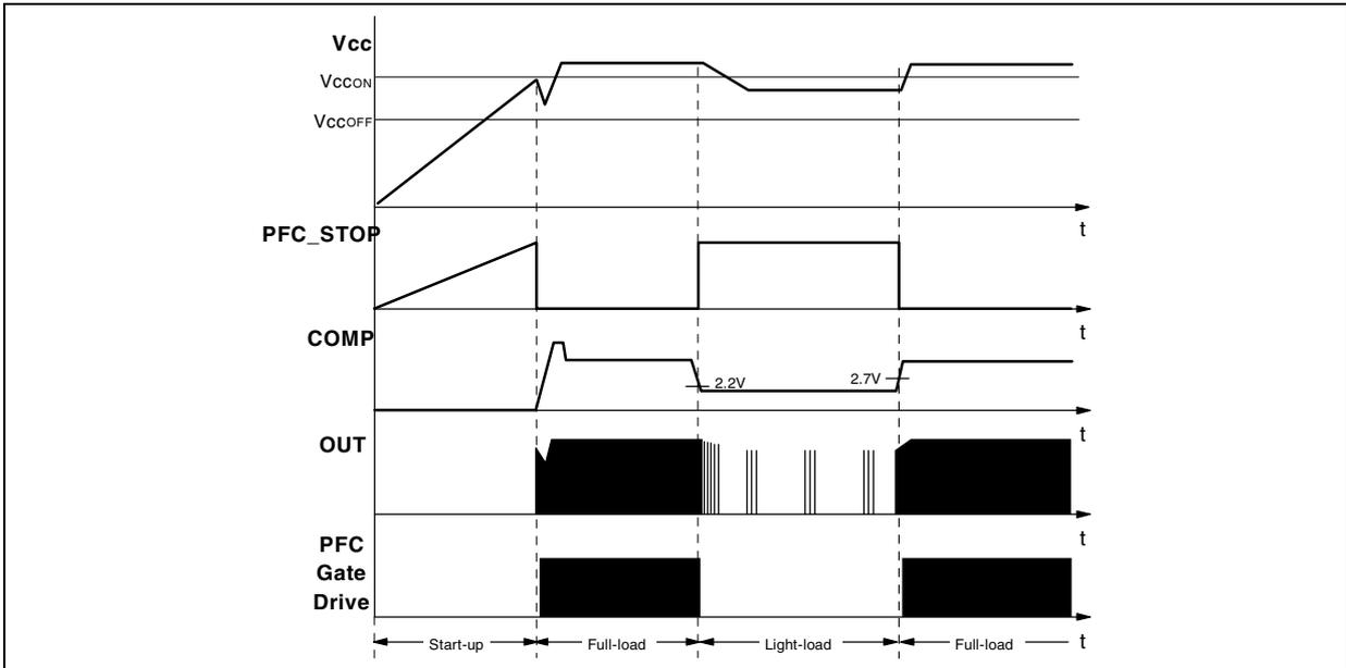
**Figure 44. Operation after DIS pin activation: timing diagram**
