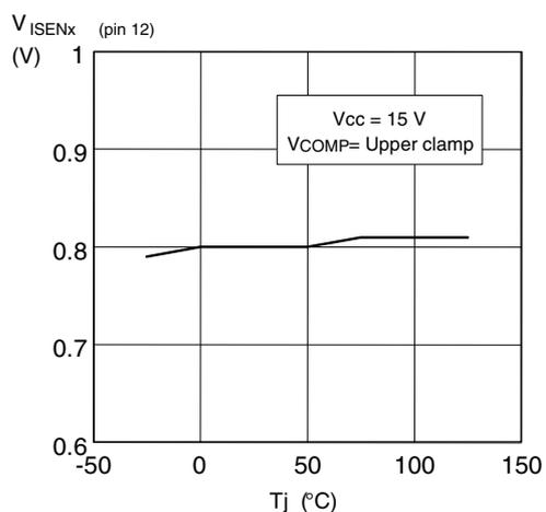
Figure 22. PFC\_STOP open/low thresholds on VCOMP vs. Tj
