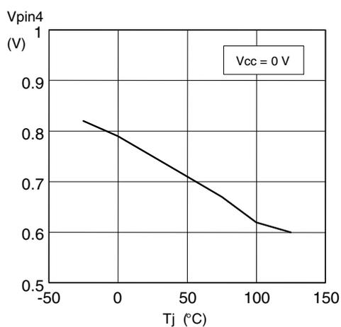
Figure 33. Gate-drive output high saturation
