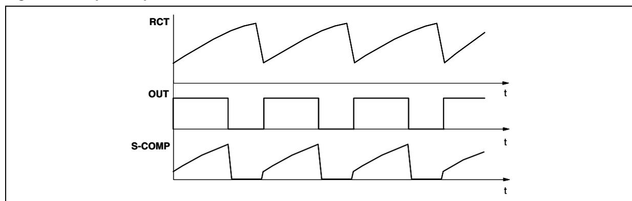
The compensation will be realized by connecting a programming resistor between this pin and the current sense input (pin 12, ISEN). The pin has to be connected to the sense resistor with another resistor to make a summing node on the pin.
