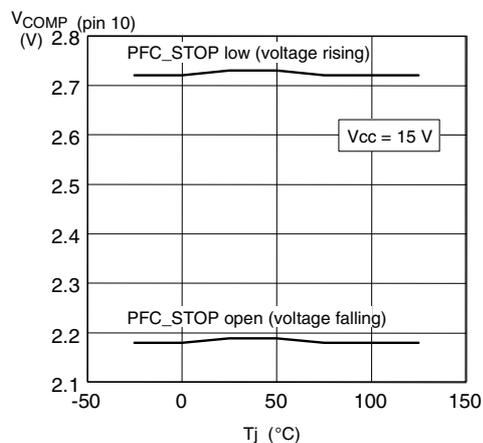
Figure 23. Standby thresholds vs. Tj
