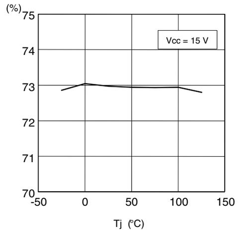
Figure 17. Oscillator frequency vs. Tj
