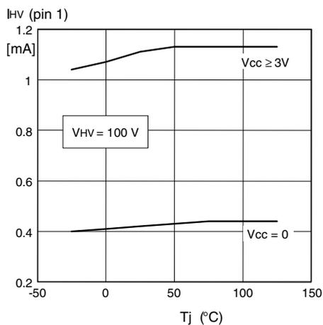
Figure 8. High-voltage generator start voltage vs. Tj
