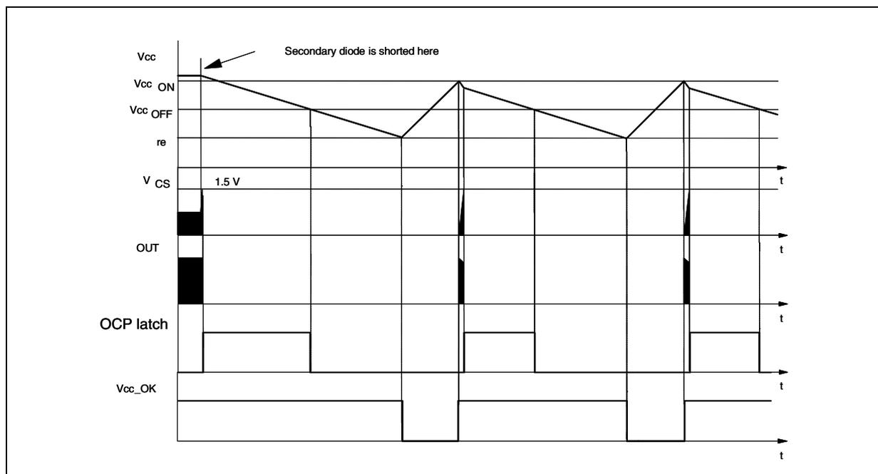
A second comparator senses the voltage on the current sense input and shuts the IC down if the voltage at the pin exceeds 1.5 V. Such an anomalous condition is typically generated by either a short circuit of the secondary rectifier or a shorted secondary winding or a saturated flyback transformer.
