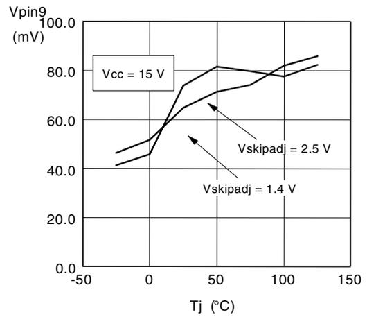
Figure 24. Standby pin dropout vs. Tj
