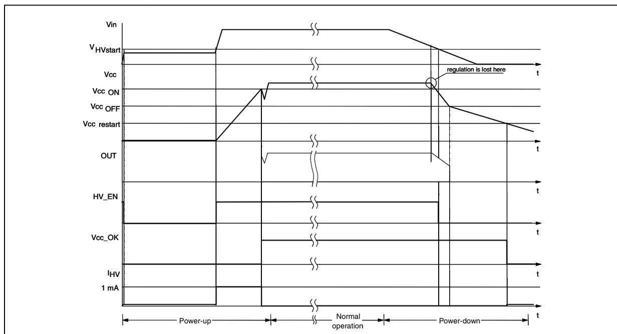
As the  $V_{cc}$  voltage reaches the start-up threshold (13.5V typ.) the low-voltage chip starts operating and the HV generator is cut off by the  $V_{cc\_OK}$  signal asserted high. The IC is powered by the energy stored in the  $V_{cc}$  capacitor until the self-supply circuit (typically an auxiliary winding of the transformer and a steering diode) develops a voltage high enough to sustain the operation.
