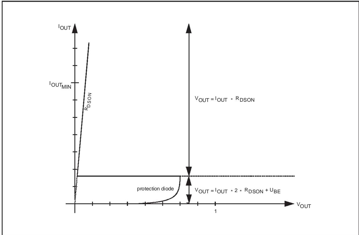
Figure 4. Output signal shape related to output current.
