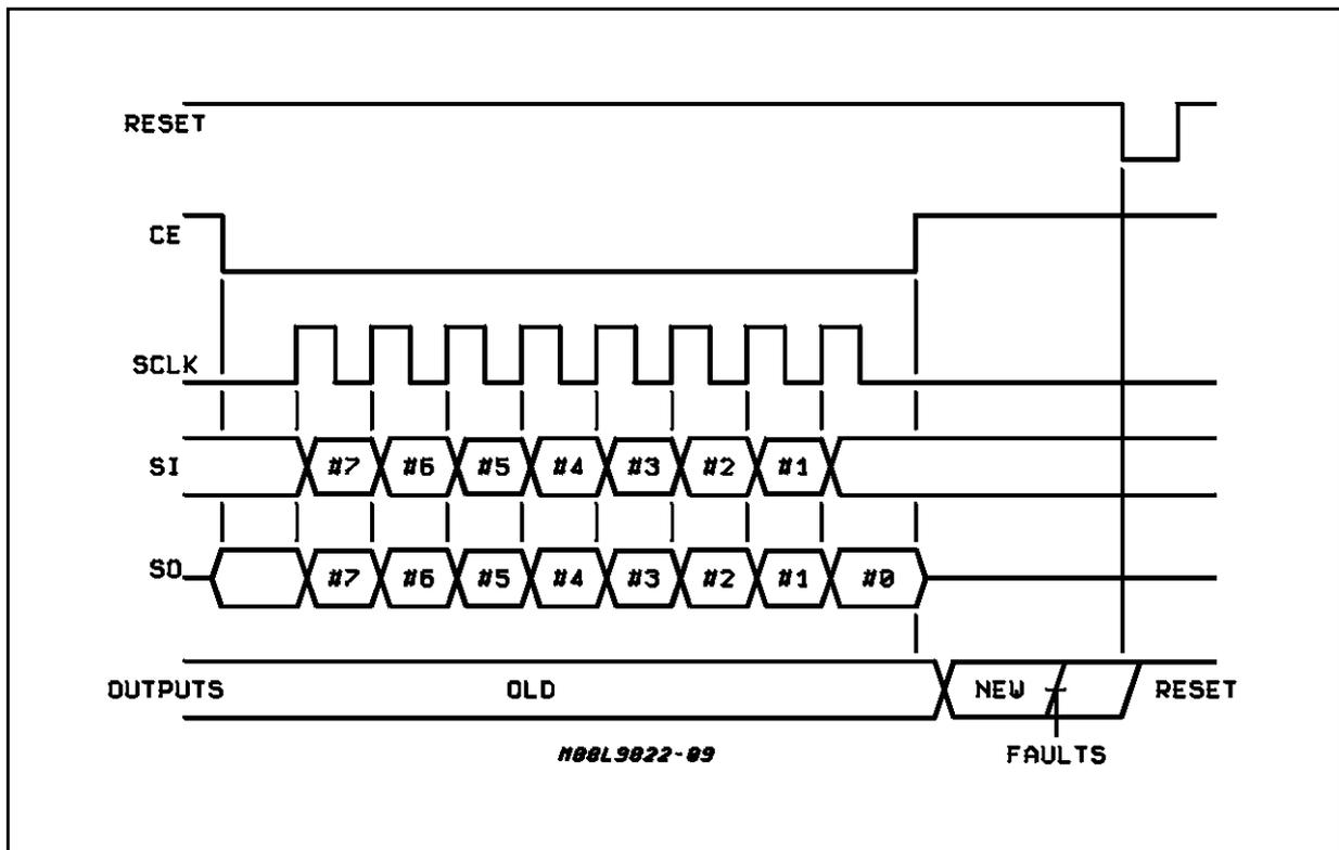
Figure 2 : Timing Diagram.
