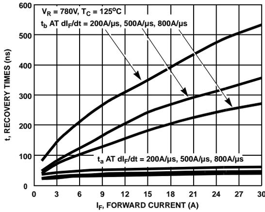
Figure 3.  $t_a$  and  $t_b$  Curves vs Forward Current
