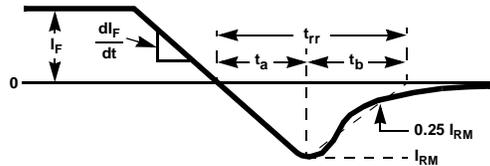
Figure 14.  $t_{rr}$  Waveforms and Definitions
