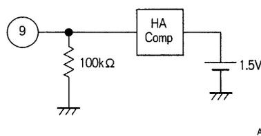
GND < pin 9 level - DC < 1.5 V: SP mode
