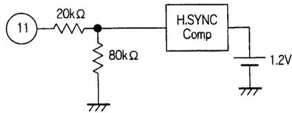
Pin 11 level - DC > 1.5 V: H-SYNC interval
