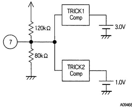
GND < pin 7 level - DC < 1.0 V: TRICK2
