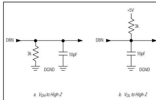
Figure 2. Load Circuits for Data-Hold Time Test
