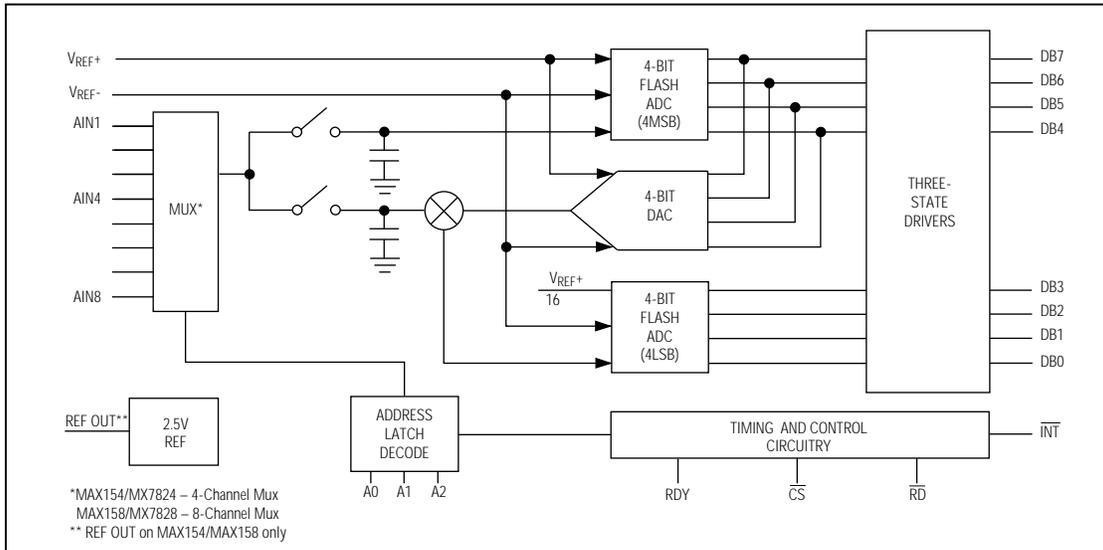
Figure 3. Functional Diagram
