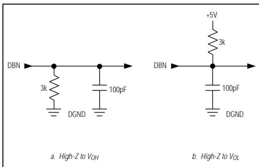
Figure 1. Load Circuits for Data-Access Time Test
