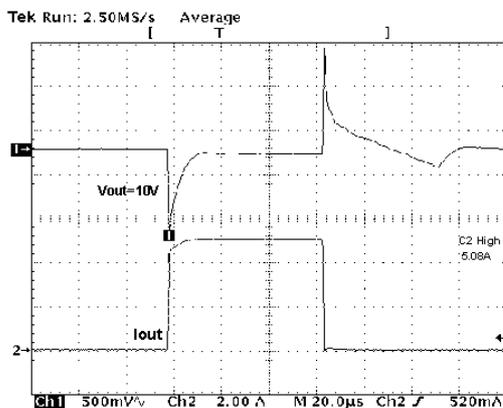
$V_I=15 V$ ,  $I_O=0.1$  to  $5 A$ ,  $C_I = 1\mu F$ (tant),  $C_O=10\mu F$ (tant), No  $C_{ADJ}$
