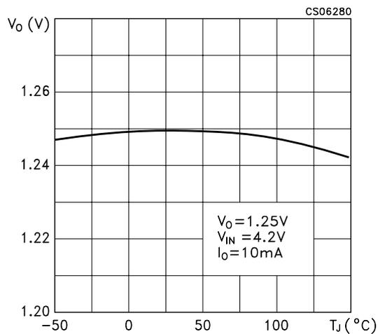
Figure 17 : Line Regulation vs Temperature
