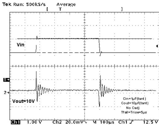
$V_I=12$  to  $13V$ ,  $I_O=200mA$ ,  $C_I = 1\mu F$ (tant),  $C_O=10\mu F$ (tant), No  $C_{ADJ}$
