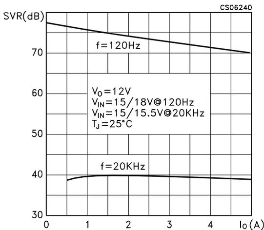
**Figure 12 : Supply Voltage Rejection vs Frequency**
