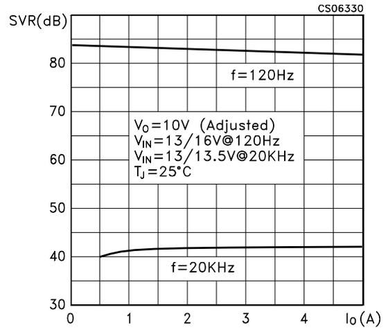
**Figure 20 : Supply Voltage Rejection vs Frequency**
