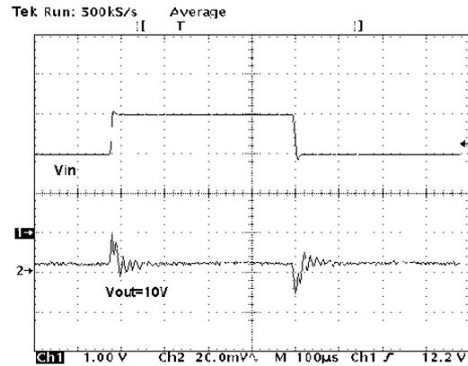
$V_I=12$  to  $13V$ ,  $I_O=200mA$ ,  $C_I = 1\mu F$ (tant),  $C_O=10\mu F$ (tant),
