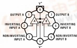
Pin 4 connected to case
