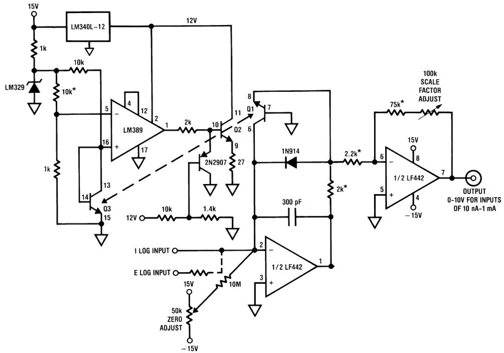
Q1, Q2, Q3 are included on LM389 amplifier chip which is temperature-stabilized by the LM389 and Q2-Q3, which act as a heater-sensor pair. Q1, the logging transistor, is thus immune to ambient temperature variation and requires no temperature compensation at all.
