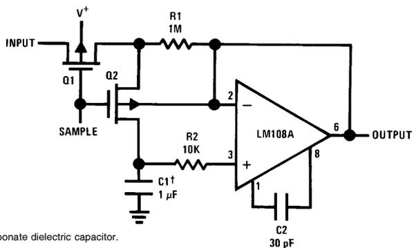
†Teflon, polyethylene or polycarbonate dielectric capacitor.
