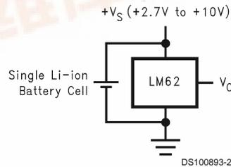
$$V_O = (+15.6 \text{ mV/}^\circ\text{C} \times T^\circ\text{C}) + 480 \text{ mV}$$
