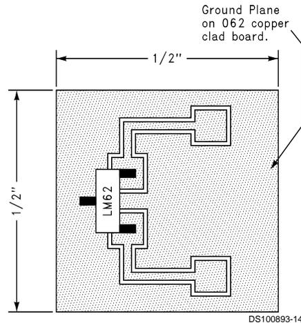
**FIGURE 2. Printed Circuit Board Used for Heat Sink to Generate All Curves.**
