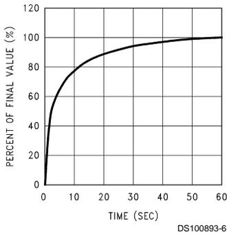
**Thermal Response in Still Air without a Heat Sink**
