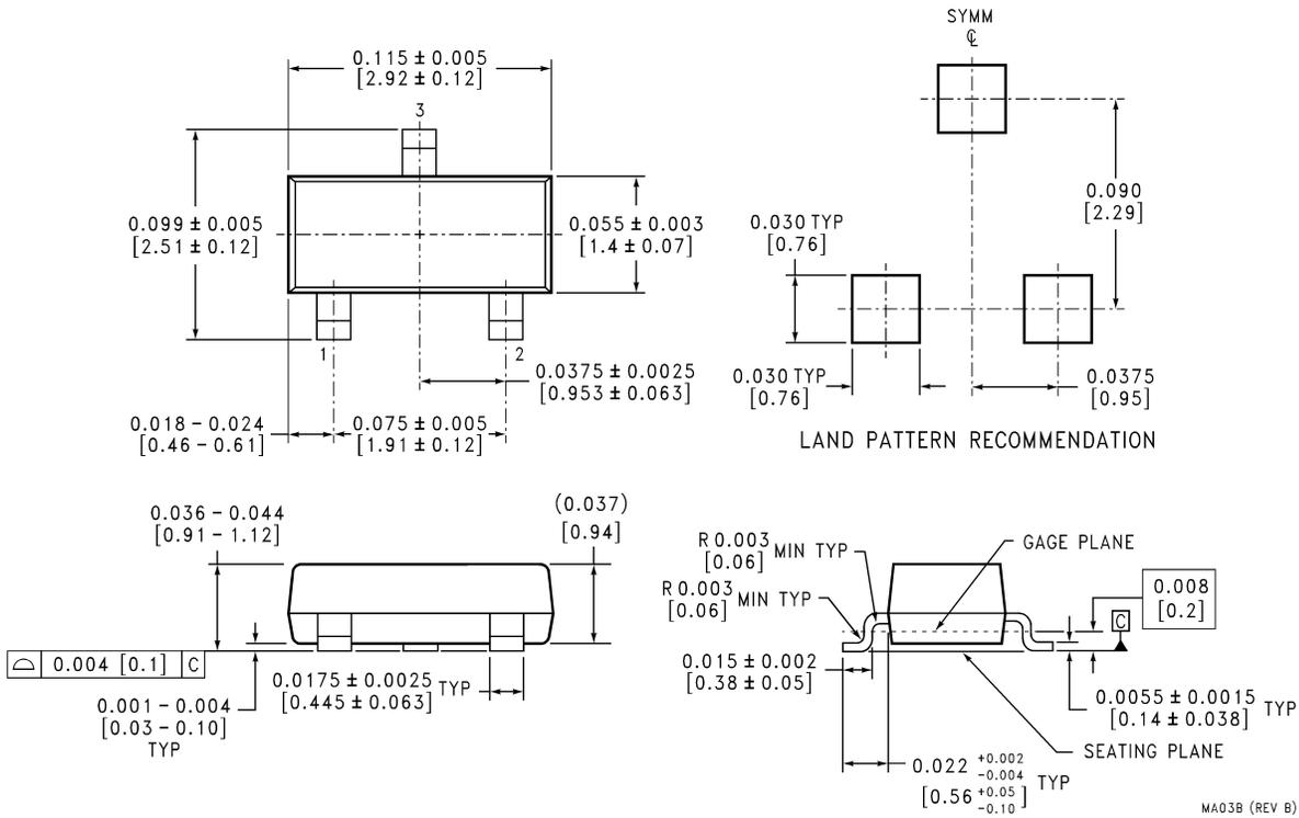
**SOT-23 Molded Small Outline Transistor Package (M3)**
