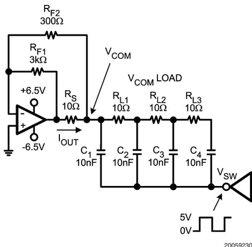
FIGURE 5.  $V_{COM}$  Driver Test Circuit
