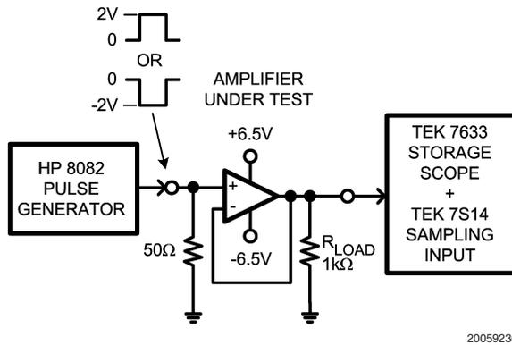
FIGURE 11. Gamma Buffer Settling Time Test Circuit
