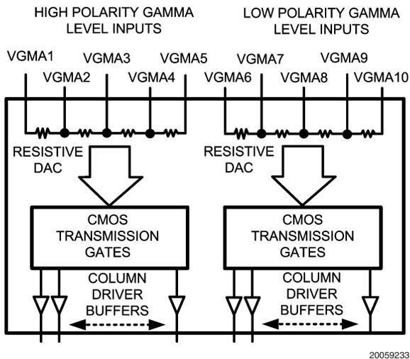
**FIGURE 8. Simplified Schematic of Column Driver IC**
